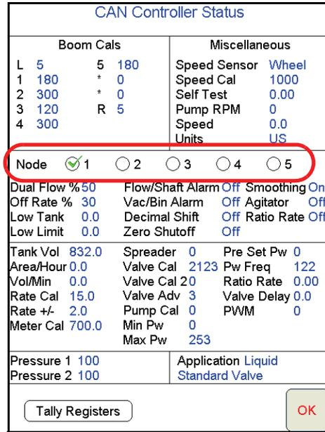
2. On the CAN Controller Status screen, select the node number for the product which the Valve Advance feature will be used.
