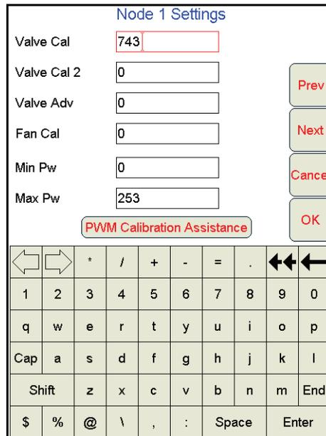
4. Use the on-screen keyboard to set the desired Valve Advance value.
