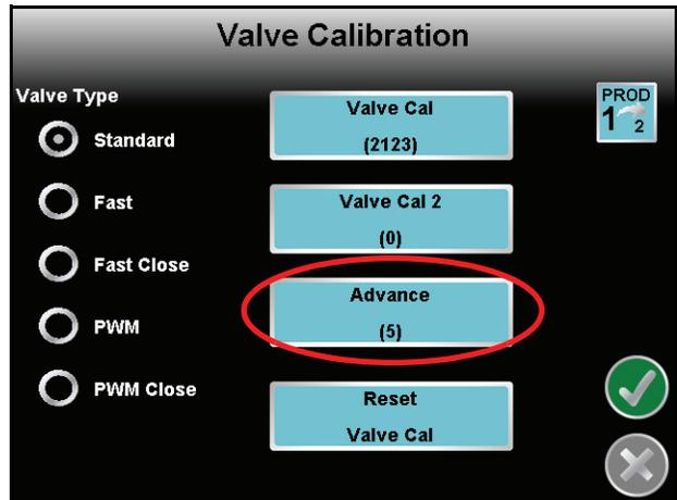
3. Use the on-screen keypad to enter the desired Valve Advance value.
