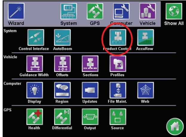
2. Touch the Valve Cal button on the Product Control Configuration screen and select the Advance button on the Valve Calibration screen.
