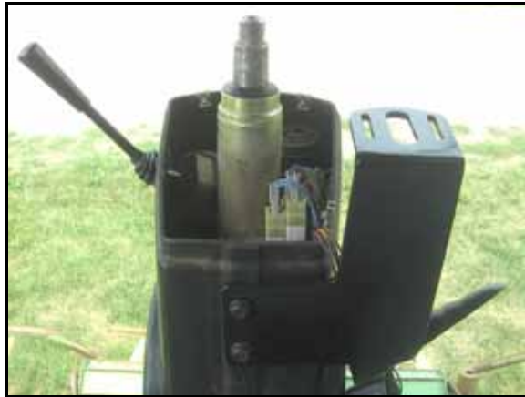
FIGURE 7. Anti-Rotation Bracket Installed
