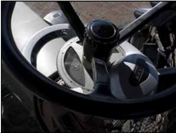
FIGURE 18. Mechanical Drive Installed
