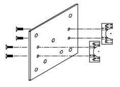
2. Secure mounting bracket to back of Viper using 4 spacers, 4 lock washers, and 4 bolts.
