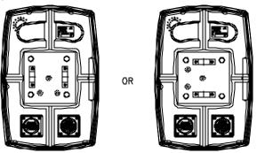
4. Secure Viper to mounting post (not included) using 2 thru-hole clamp halves and 4 knobs.
