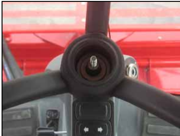
FIGURE 5. Steering Wheel Nut Removed
