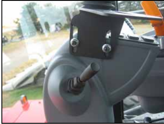
FIGURE 13. Anti-Rotation Bracket Installed
