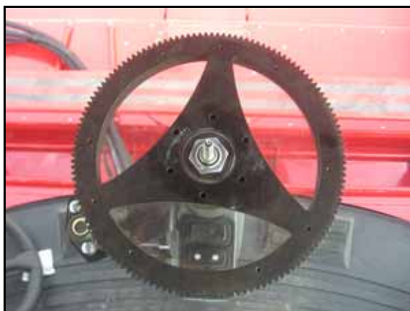
FIGURE 17. Ring Gear Assembly Installed
