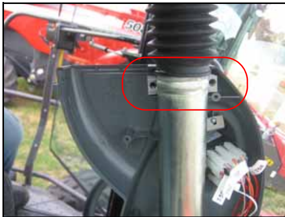
FIGURE 9. Threaded Half of Auto-Rotation Collar Placement on Console Cover
