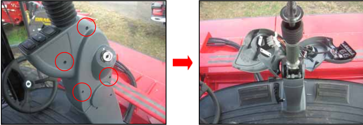
FIGURE 8. Console Cover Screws Removed
