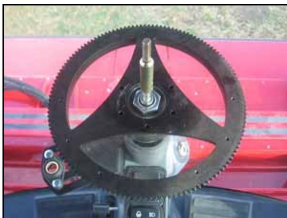
FIGURE 18. Telescope Adapter Assembly Installed
