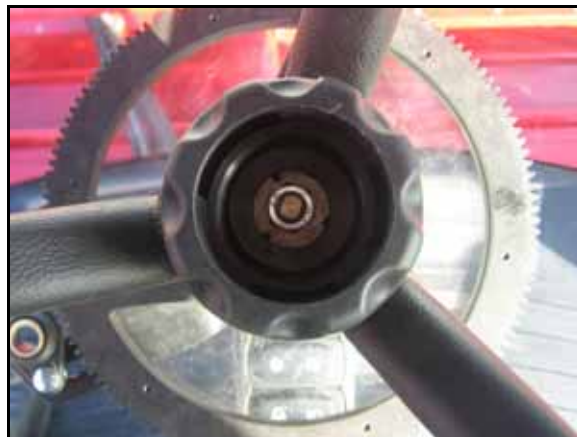
FIGURE 22. Telescope Knob Reinstalled
