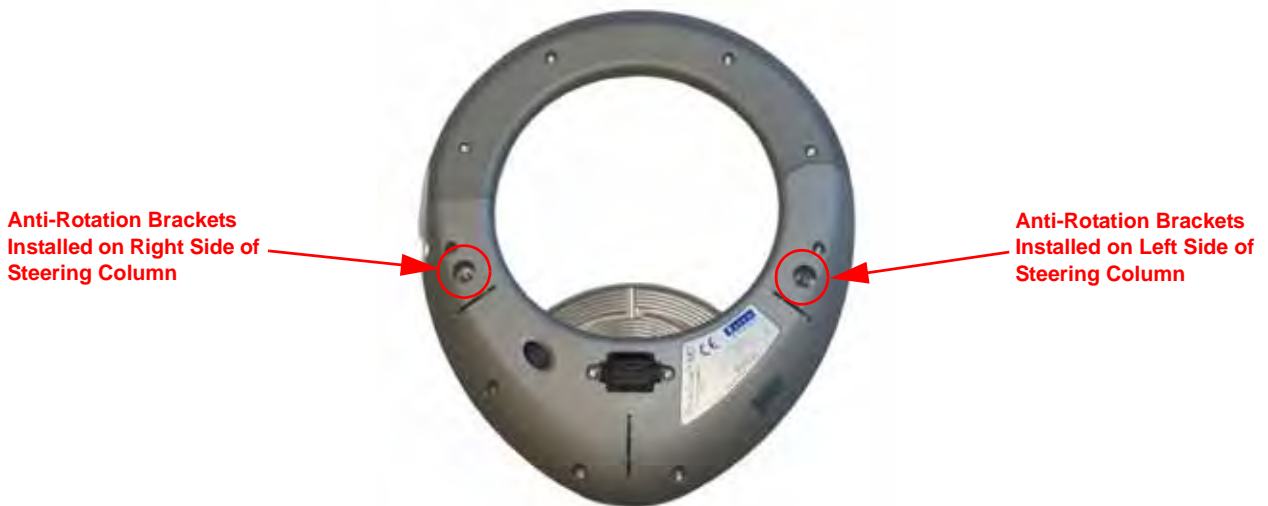
FIGURE 24. Anti-Rotation Pin Installation Locations
