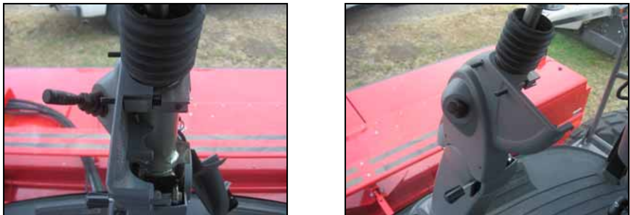
FIGURE 11. Anti-Rotation Collar Assembly Installed
