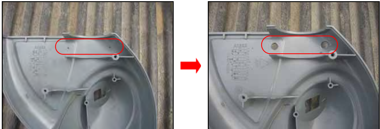
FIGURE 10. Holes Drilled in Console Cover
