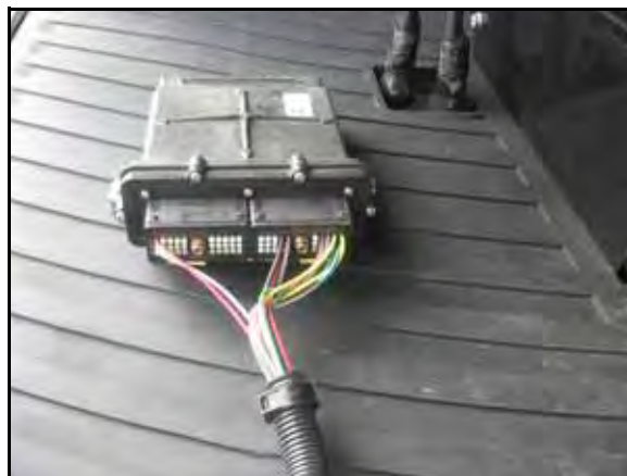
FIGURE 5. Node Harness Installed on SmarTrax Node
