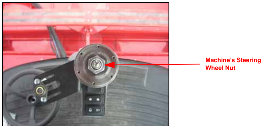
FIGURE 16. Machine's Steering Wheel Nut Reinstalled
