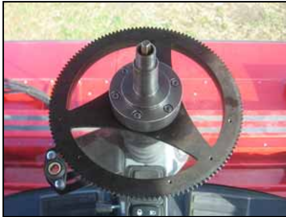
FIGURE 19. Male Spline Adapter Installed
