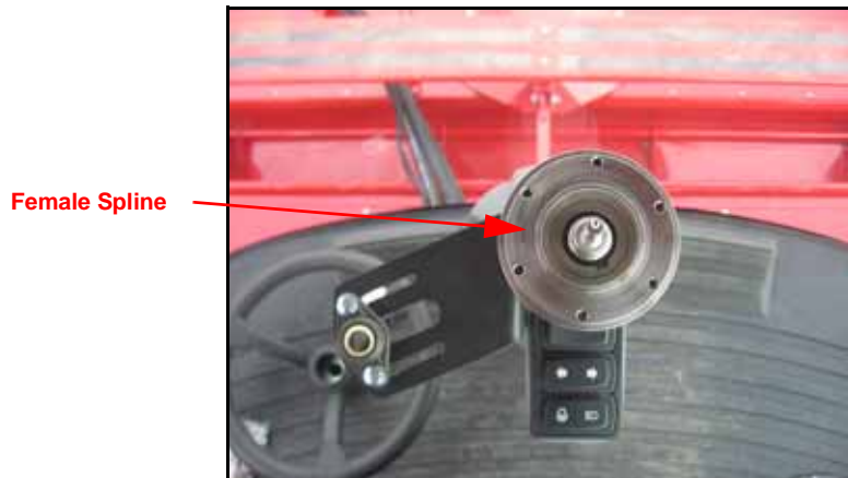
FIGURE 15. Female Spline installed on Machine's Steering Column
