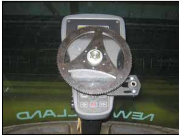
FIGURE 9. Ring Gear Assembly Installed
