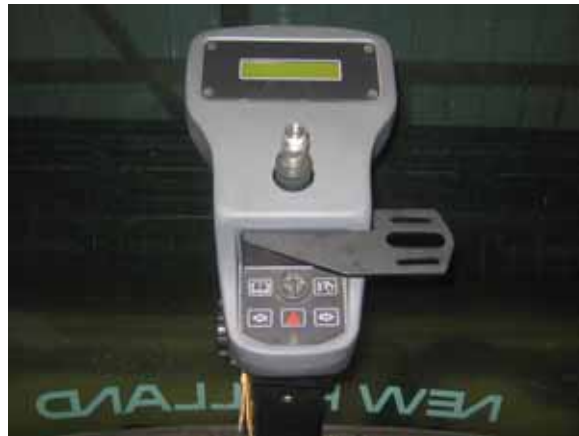
FIGURE 6. Anti-Rotation Bracket Installed
