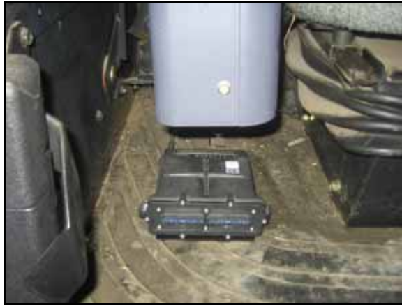
FIGURE 2. SmarTrax MD Node Installed
