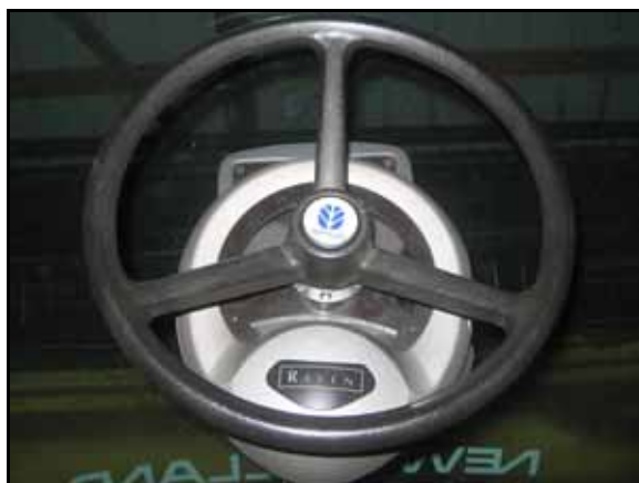
FIGURE 16. Mechanical Drive Installed
