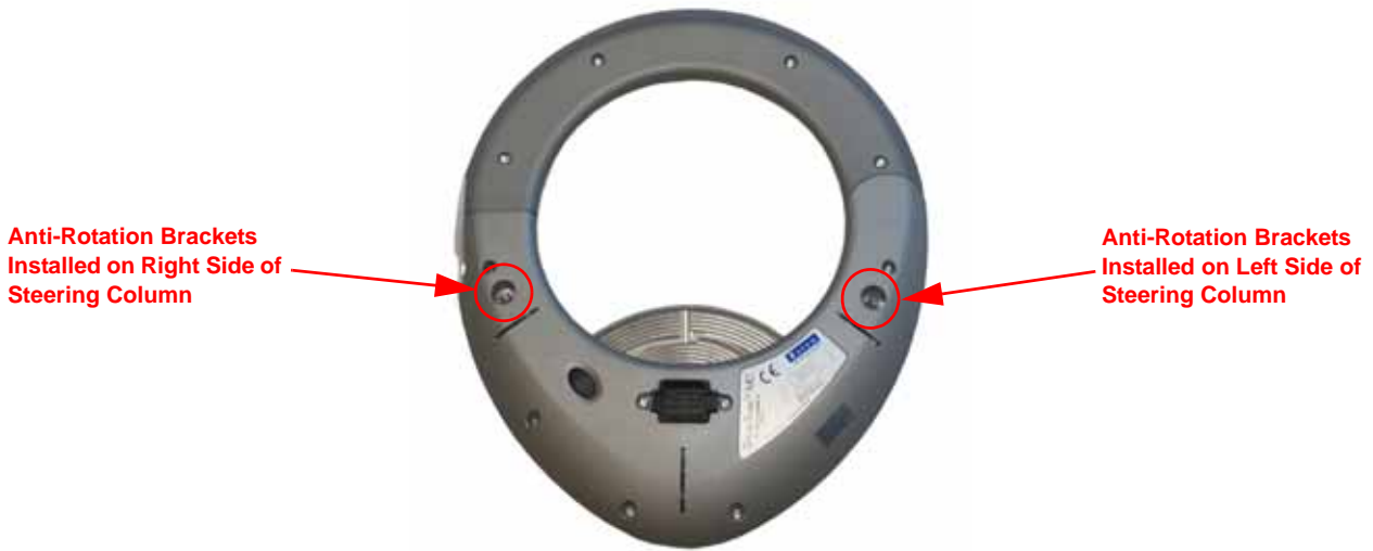
FIGURE 15. Anti-Rotation Pin Installation Locations
