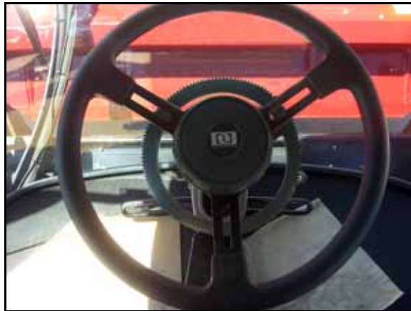
FIGURE 12. Machine's Steering Wheel Cap Reinstalled
