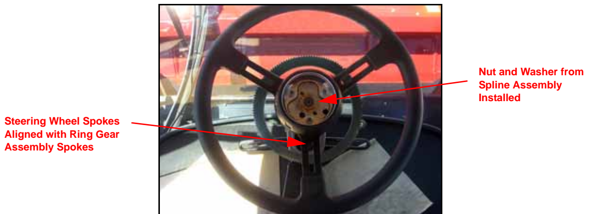
FIGURE 10. Steering Wheel Installed on Ring Gear Assembly
