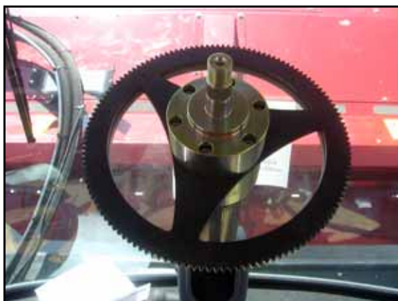
FIGURE 8. Male Spline Assembly Installed
