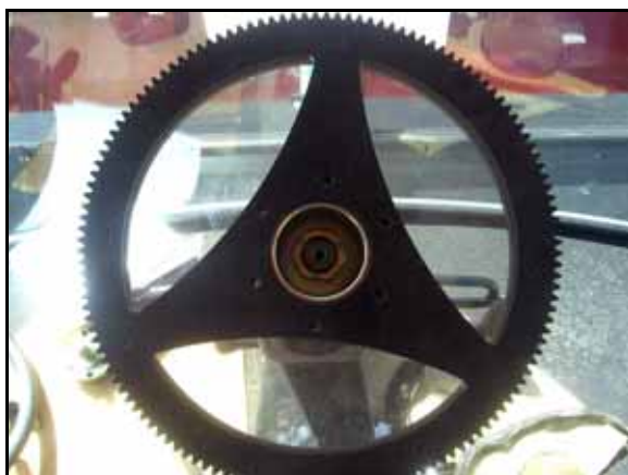
FIGURE 7. Ring Gear Assembly Installed
