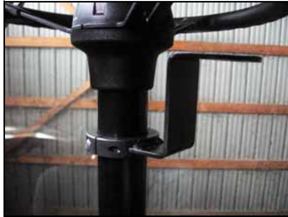
FIGURE 13. Anti-Rotation Bracket Installed
