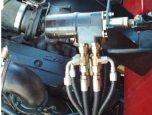
Hose connection to orbital tee fitting
