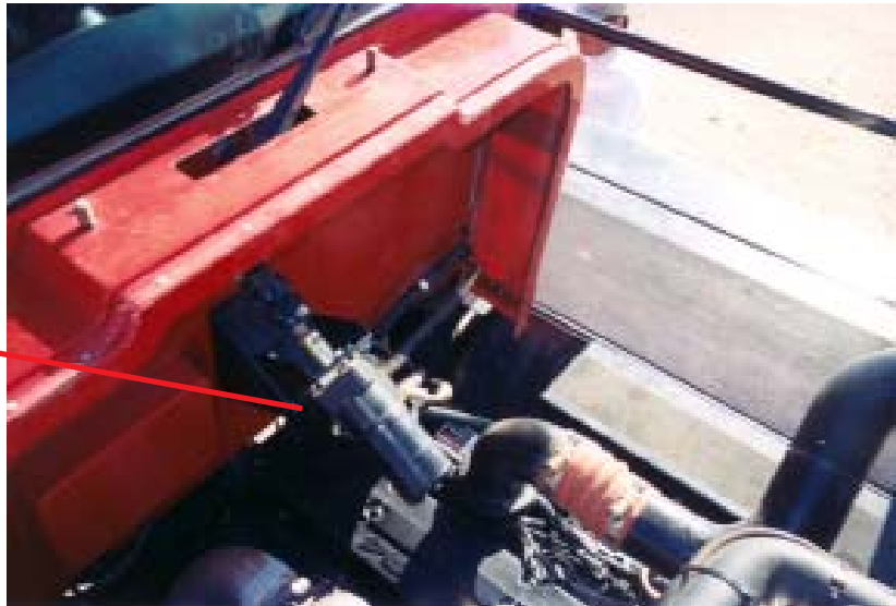
LS-STEER Line connection point to steering orbital
