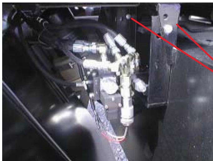
Hole locations for hydraulic bracket
