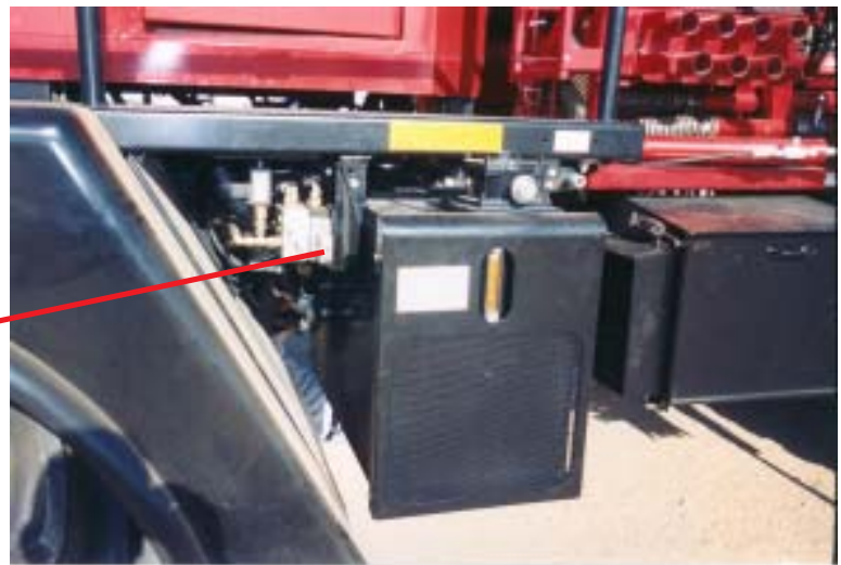
Mounting Location for Hydraulic Valve
