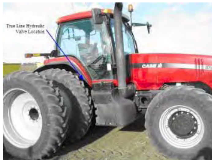
Steering Assist Valve Bank mounting location
