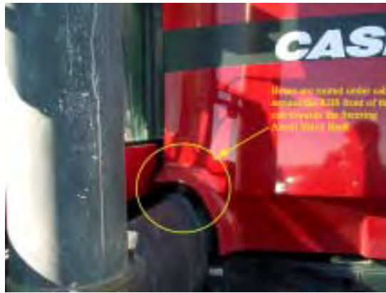
Hose routing under cab
