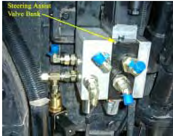
Steering Assist Valve Bank & Pressure Switch (NOTE: Valve in picture differs from one currently used.)
