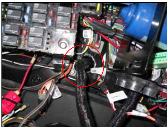
FIGURE 6. Node Harness Routed to Machine's Bulkhead
