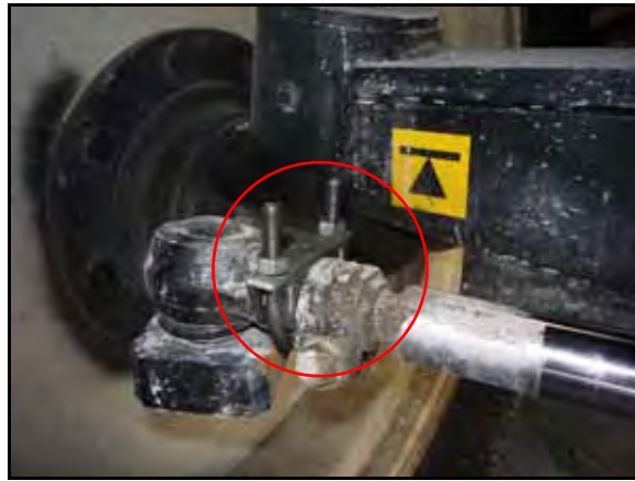
FIGURE 8. Clamps Installed on Rod-End of Steering Cylinder
