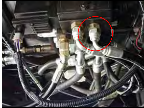
FIGURE 11. Hydraulic Hose Installed on SmarTrax Valve
