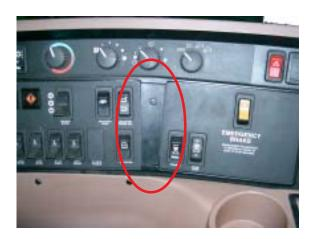
Remove screw and retainer plate.
