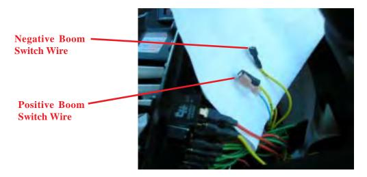
c. Route the two smaller wire bundles from the Smartboom Cable P/N 115-1001-027 up into the switch location.
