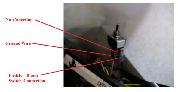
c. Attach supplied insulating terminals to remaining empty posts on switch.
