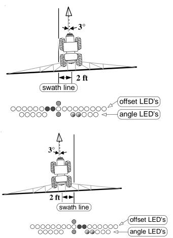
In the diagram shown to the left, the machine is 2 feet right of the swath line and has the same angle alignment as previously. The two offset LED's on the left are telling the operator to drive to the left. The two angle LED's to the right are telling the operator to turn to the right. This looks like a problem. However, the operator can drive left to correct the offset error, but already knows a right turn correction will be needed very soon.
