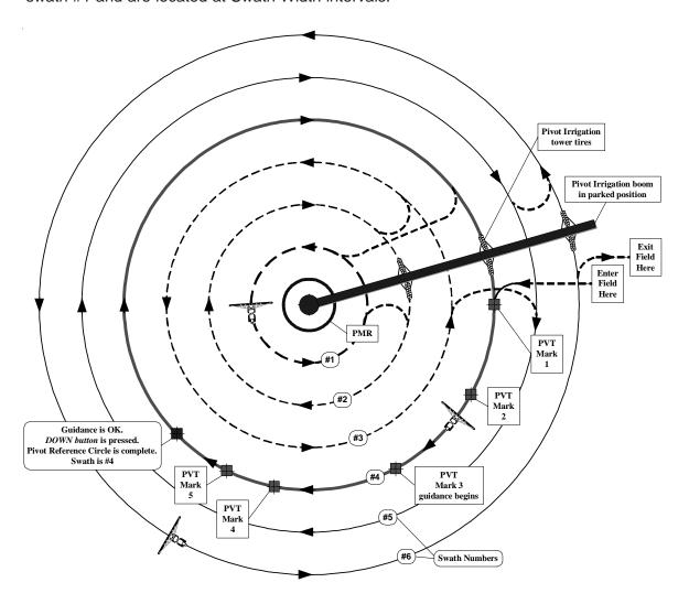
The Pivot Minimum Radius setting defines a circular area at center of the field. Circular swaths are assigned outside of this area. As the radius of circular swaths become smaller and smaller, the inside spray nozzle moves slower than the outside spray nozzle. The **PMR** setting determines the smallest circle to be sprayed. The **PMR** setting may also be used to define an unplanted area at the center of the field that is used for installed equipment or storage.
