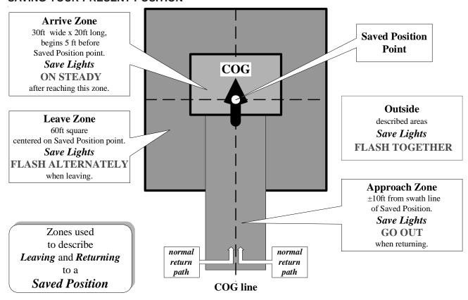
Using the Smartbar 'SAV POS' function, you can leave your current swathing position and return to it later to continue the present swathing operation. To save your current position, locate the 'SAV POS' screen on the menu and press the *SELECT button*. A position may be saved after stopping. However, do not back up prior to saving a position or the saved COG will be in the wrong direction.
