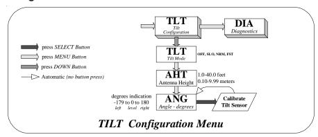
When a Smartbar has a Tilt Sensor Upgrade Option installed, a new top level configuration menu (**TLT**) is added just prior to the **DIA** top level configuration menu. Press the *DOWN button* at the **TLT** top level menu to enter the **TLT** configuration sub-menus.
