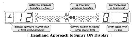
When operator is leaving a headland area and approaching the parallel swath area, the center top green LED will flash *(center bottom green LED is OFF)*. The *Headland Approach Display* shows the distance to the headland boundary, instead of the swath number. This prompts the operator to prepare to turn the applicator ON. The center top and bottom green LED's will both go ON when the operator crosses the boundary into the parallel swath area.
