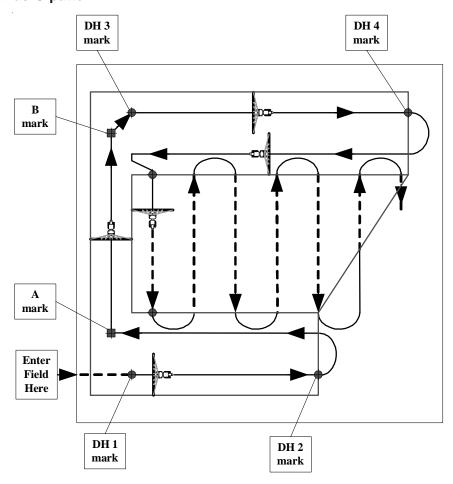
The **Double Headlands C** pattern provides parallel swathing between two straight double headland areas. Using the C pattern, swathing progresses toward an "open" end, allowing the last swath to easily align with the edge of the field. This pattern can be used with Swath Types (**SWA**) Back and Forth (**BF**) or Snap-To-Swath (**SNP**) and uses the direction (**DIR**) control **AUT/MAN** setting to determine the layout of the C pattern.
