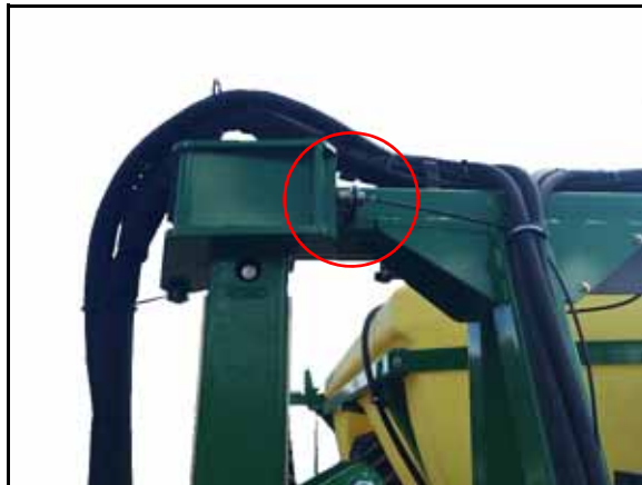
FIGURE 9. Proximity Switch Installed (Near Right Wing Folding Joint on Center Section)
