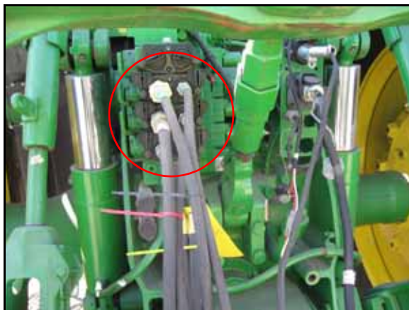
FIGURE 2. Machine's Selective Control Valve
