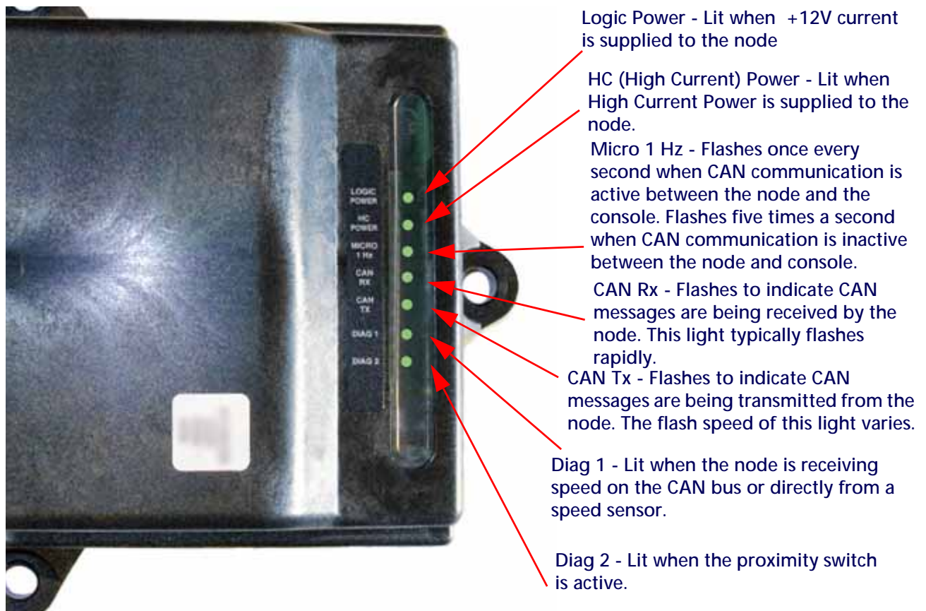
FIGURE 1. CAN Control Node LEDs
