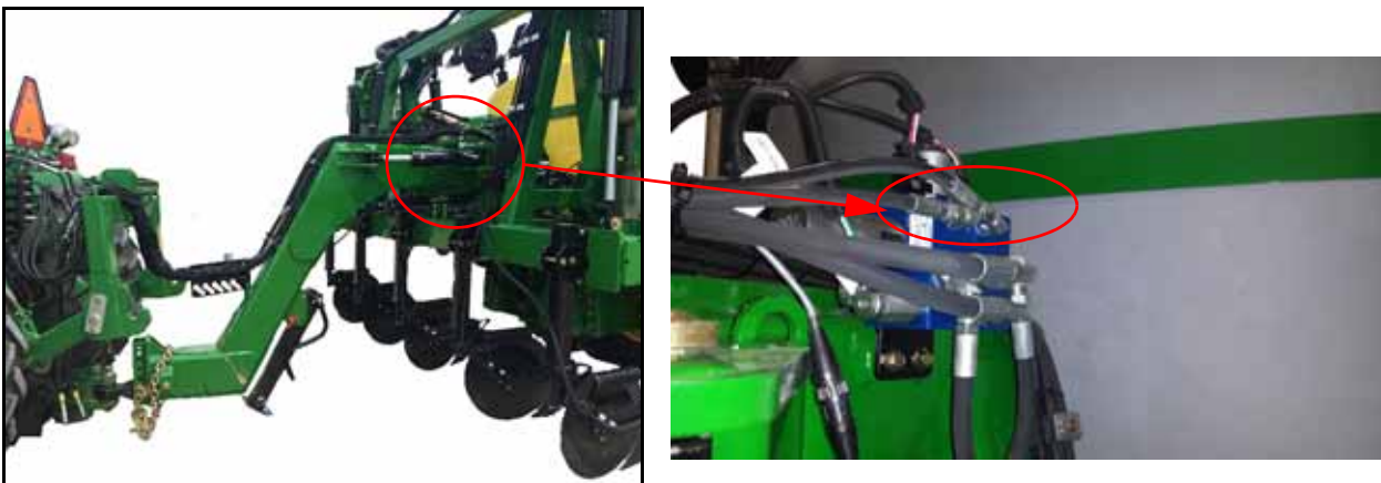
FIGURE 4. Left and Right Steering Hoses Installed
