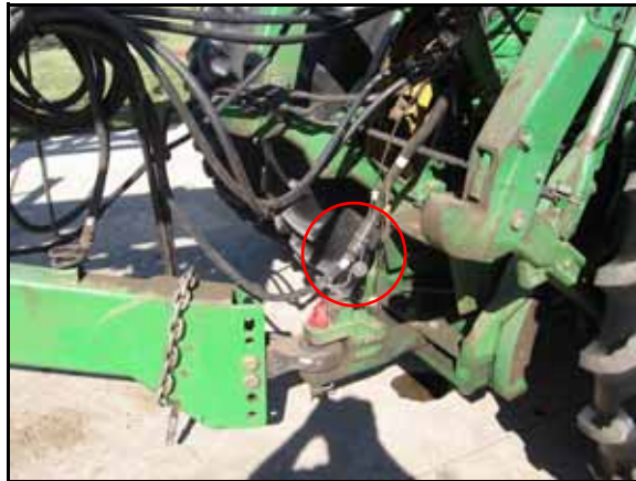
FIGURE 1. Steerable Hitch Harness Cable Installed
