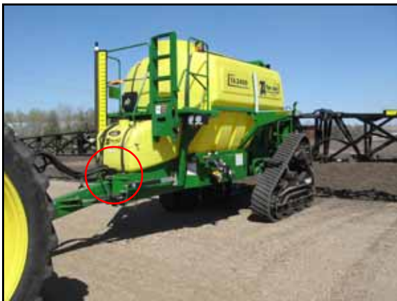
FIGURE 8. Rotary Sensor Installed
