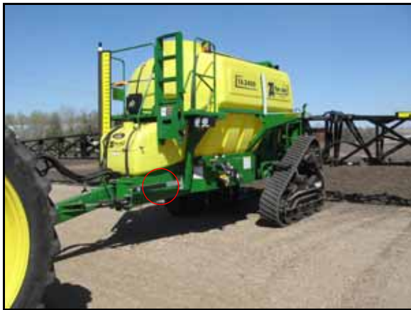
FIGURE 1. Hydraulic Valve Installed
