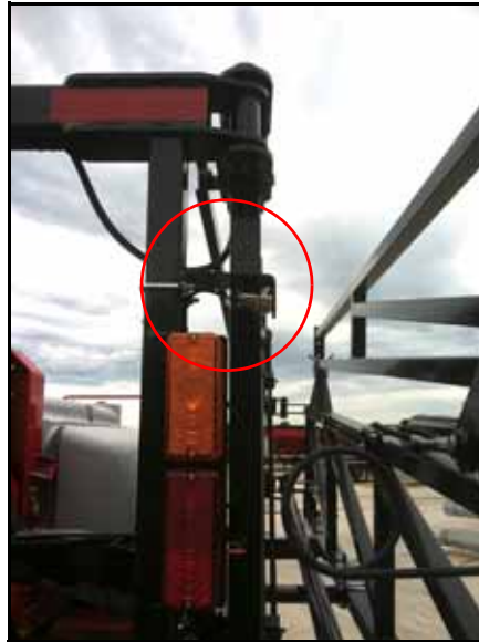
FIGURE 10. Proximity Switch Installed (Near Right Wing Folding Joint on Center Section of the Sprayer)
