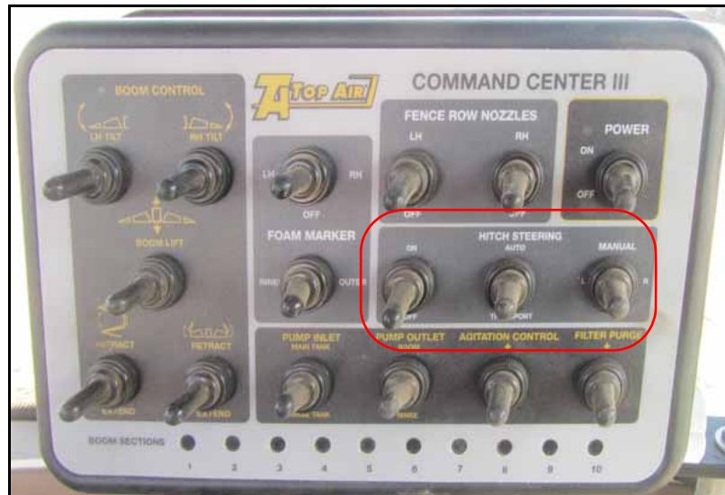
FIGURE 7. Top Air Switchbox
