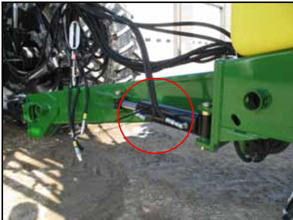
FIGURE 4. Left and Right Steering Hoses Installed
