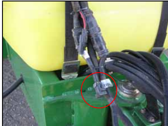
FIGURE 2. Terminator Installed on Steerable Hitch Harness
