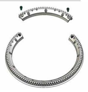
3. Install the larger section under the steering wheel around the steering column. Install with the gear teeth on the top, closest to the steering wheel. See Figure 3, "Installed Main Gear," .
