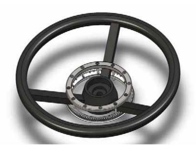
4. Tighten screws with a hex key until the main gear and ring fit snugly to the steering wheel. Tighten the screws in a cross-pattern (as opposed to tightening each screw in a clockwise or counter-clockwise order).
