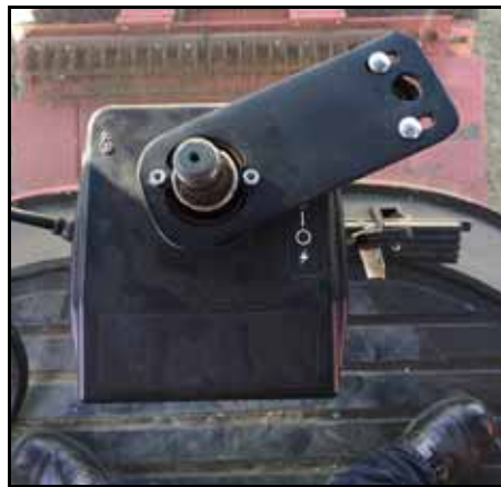
FIGURE 6. Anti-Rotation Bracket Aligned on Steering Shaft
