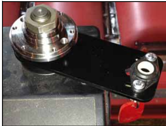
FIGURE 8. Female Spline Adapter Installed on Steering Column
