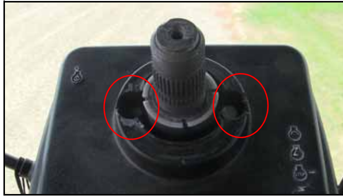
FIGURE 5. Bolts to be Removed
