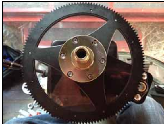
FIGURE 10. Male Spline Adapter Installed
