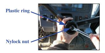
4. Remove the plastic ring by using a small flat blade screwdriver.
