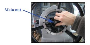
3. Tighten the nut using a wrench. This will seat the assembly onto the steering column.
