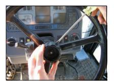
5. On most tractors, the steering wheel is attached to the steering shaft with a large nut. Loosen and remove the nut using a wrench.
