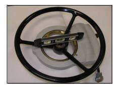
4. Once the steering wheel is level, set the supplied upper ring (6 5/16") on the steering wheel. Align the upper ring to the brass ring gear mounting holes. Fasten the upper ring to the brass ring using the
