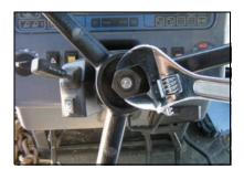
6. After the nut is removed, the steering wheel is free and should be removed. To remove the steering wheel from the steering shaft, pull the wheel manually towards you.
