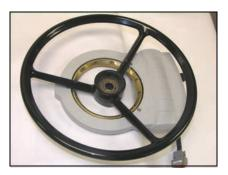
The steering wheel should be as flat as possible. Using the level over top of the steering wheel will ensure this.
