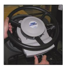
2. Once the system is engaged, release the steering wheel. The QuickTrax system will now take over steering and the steering wheel will turn and steer without any operator interventions.
