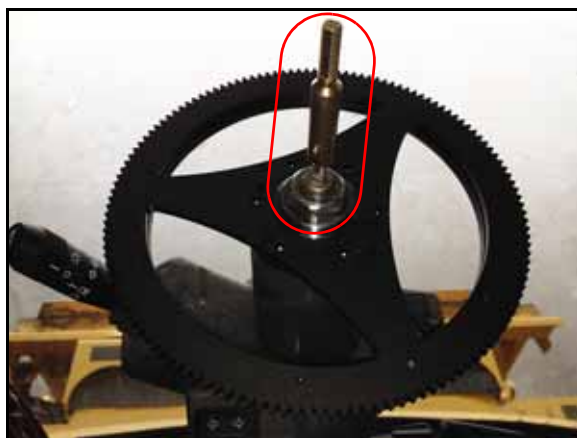
FIGURE 15. Telescope Adapter Assembly Installed
