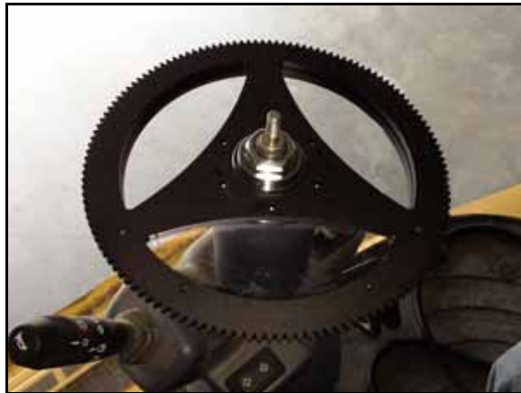
FIGURE 14. Ring Gear Assembly Installed
