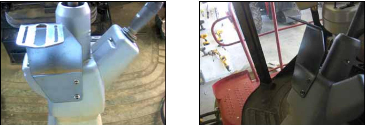
FIGURE 10. Anti-Rotation Bracket Installed
