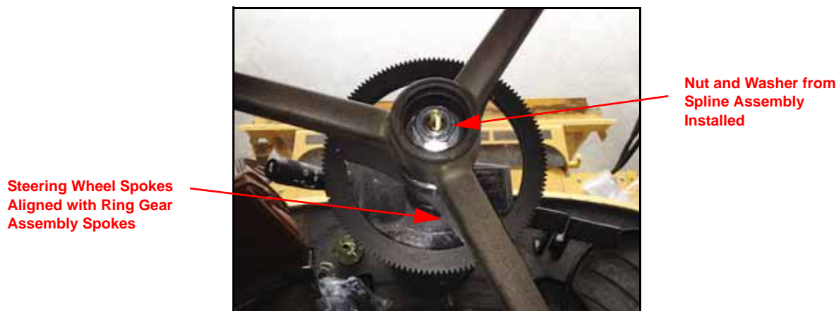
FIGURE 17. Steering Wheel Placement
