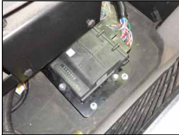
FIGURE 8. Node Harness Installed on SmarTrax Node
