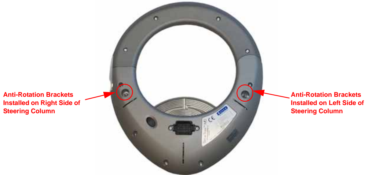
FIGURE 20. Anti-Rotation Pin Installation Locations
