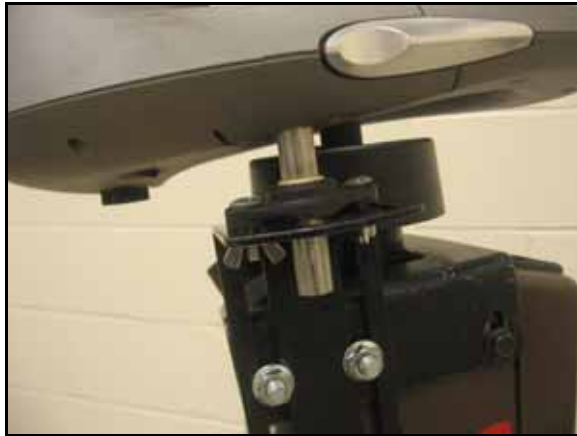
FIGURE 22. Anti-Rotation Pin Installed in Bracket Assembly
