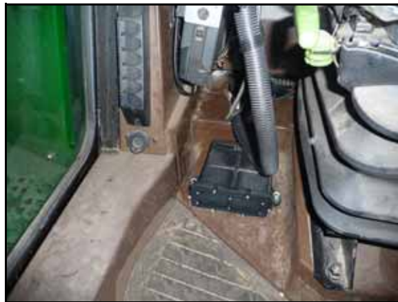
FIGURE 3. SmarTrax MD Node Installed
