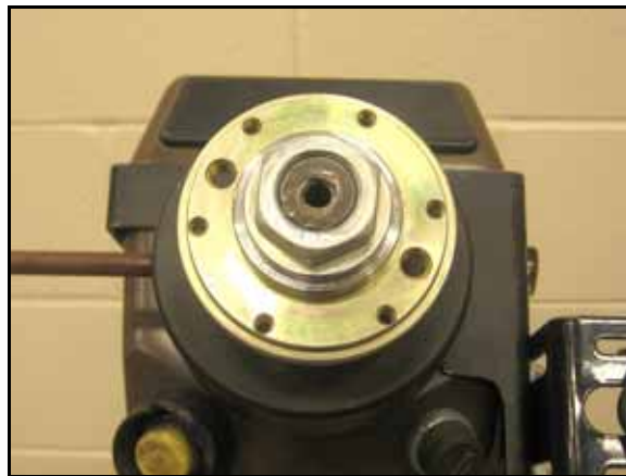
FIGURE 12. Machine's Steering Wheel Nut Installed
