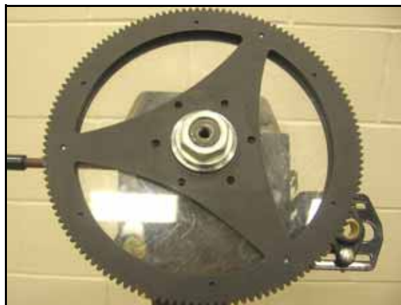
FIGURE 13. Ring Gear Assembly Installed
