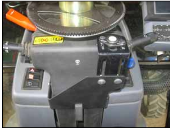
FIGURE 15. L-Shaped Bracket Installed
