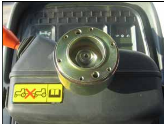
FIGURE 6. Machine's Steering Wheel Nut Installed
