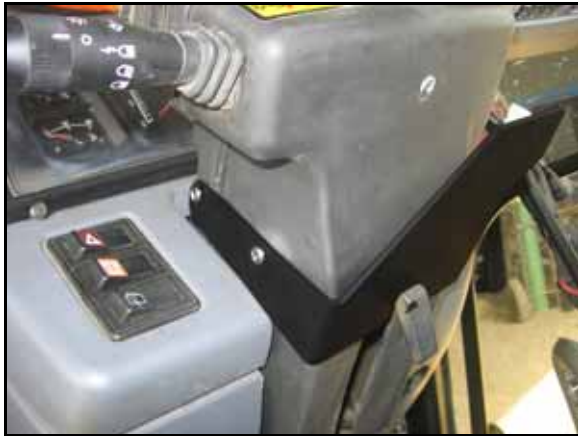
FIGURE 13. U-Shaped Anti-Rotation Bracket Installed
