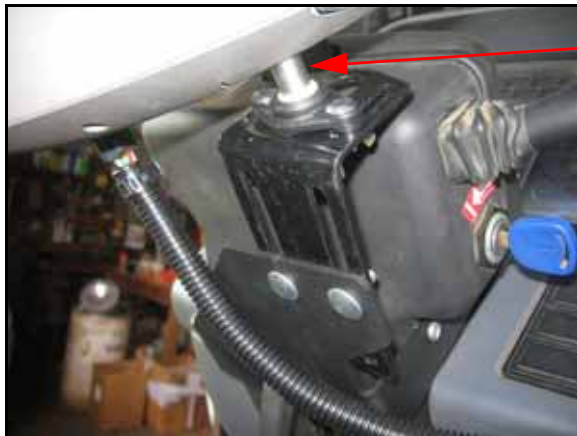
FIGURE 17. Anti-Rotation Pin Installed in Bracket Assembly
