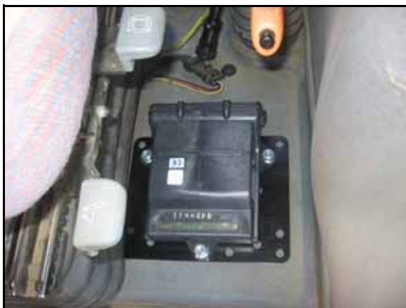
FIGURE 3. SmarTrax MD Node Installed
