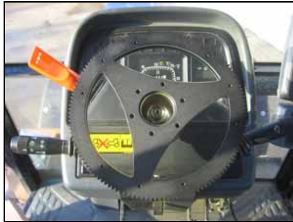
FIGURE 7. Ring Gear Assembly Installed
