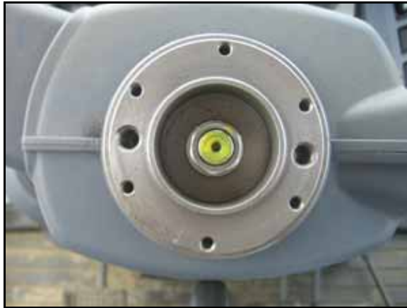
FIGURE 8. Machine's Steering Wheel Nut Installed
