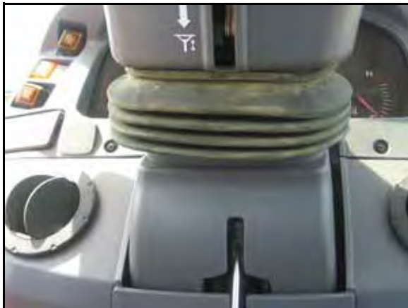
FIGURE 14. Anti-Rotation Collar Bracket Installation Location
