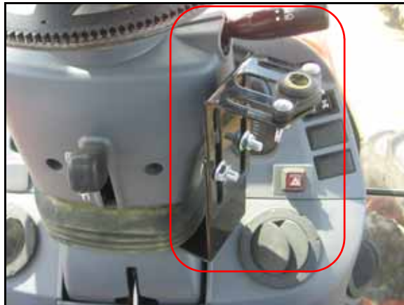
FIGURE 16. L-Shaped Anti-Rotation Bracket Installed
