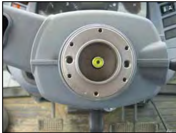
FIGURE 7. Female Spline Adapter Installed on Steering Column
