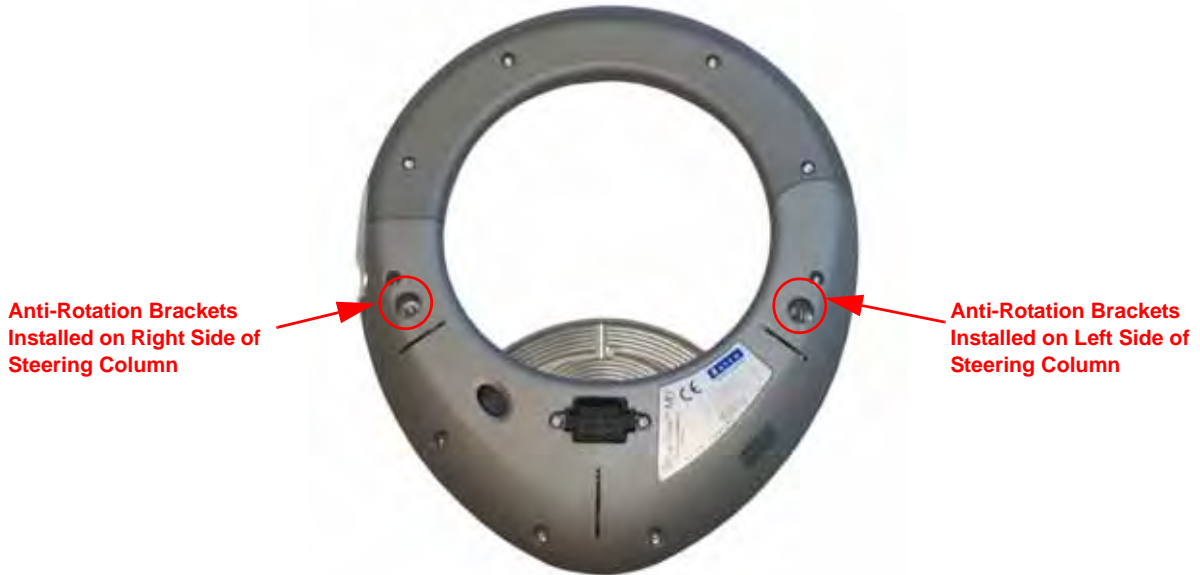
FIGURE 21. Anti-Rotation Pin Installation Locations
