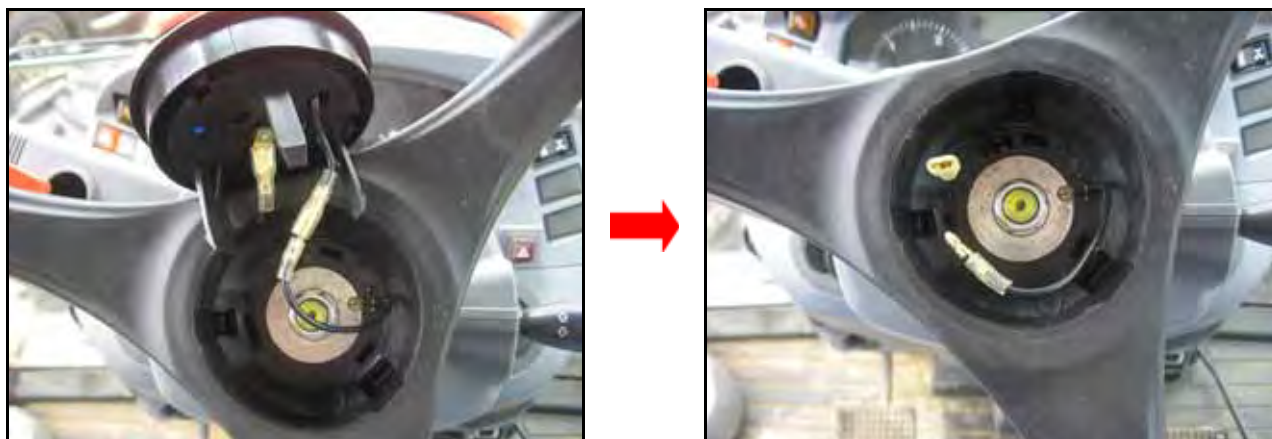
FIGURE 3. Horn Switch Disconnected
