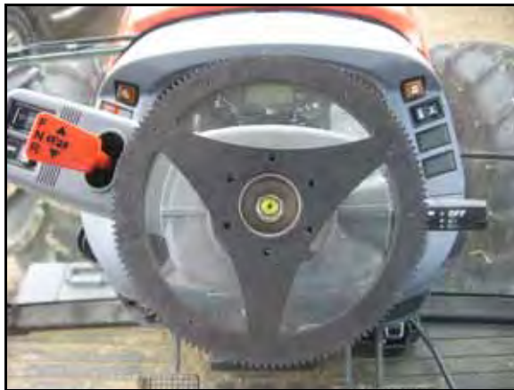
FIGURE 9. Ring Gear Assembly Installed
