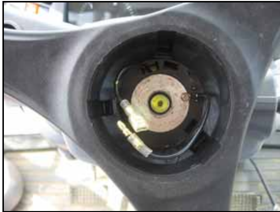
FIGURE 4. Machine's Steering Wheel Nut Removed
