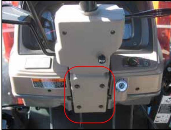
FIGURE 17. Anti-Rotation Bracket Mounting Location
