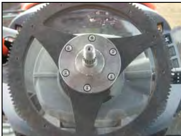
FIGURE 10. Male Spline Adapter Assembly Installed
