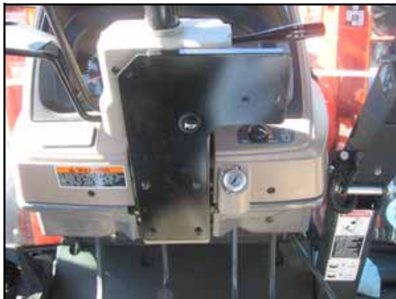
FIGURE 18. Anti-Rotation Bracket Installed
