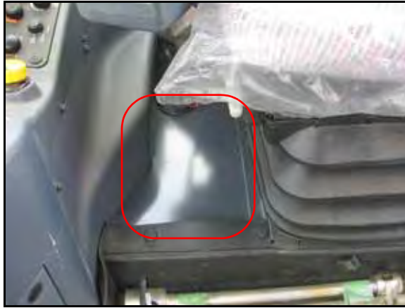
FIGURE 2. SmarTrax MD Node Mounting Location
