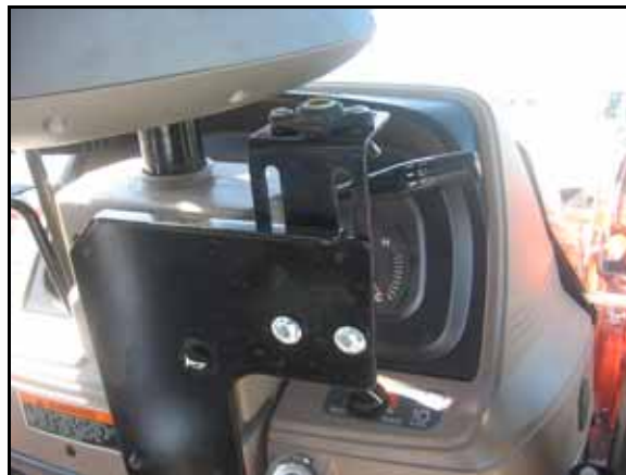
FIGURE 20. L-Shaped Bracket Installed
