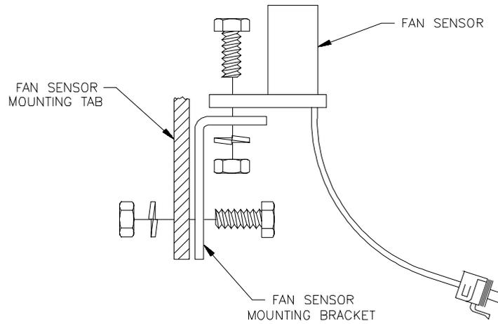
Assemble Fan Sensor to fan sensor bracket with stainless steel bolt, lock washer, and nut. Assemble fan sensor bracket to fan sensor mounting tab on box with stainless steel bolt, lock washer, and nut. (See Figure above).
