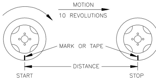
**NOTE:** This measurement is critical to the performance of the Console. **MEASURE CAREFULLY.** Be sure tire is properly inflated before measuring. Measure tire in type of soil in which you will be spraying. Circumference of tire will vary when measured in soft soil versus hard packed soil. For best results, measure several times and average the results.
