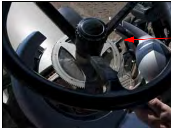
FIGURE 18. Anti-Rotation Pin Installed in Bracket Assembly
