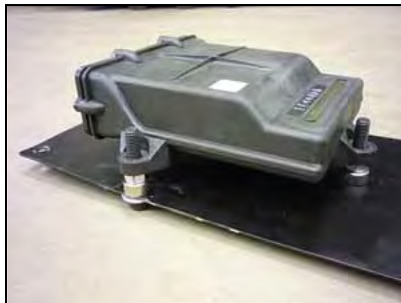
FIGURE 3. Node Installed on Steel Plate
