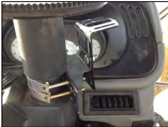
FIGURE 15. L-Shaped Bracket Installed
