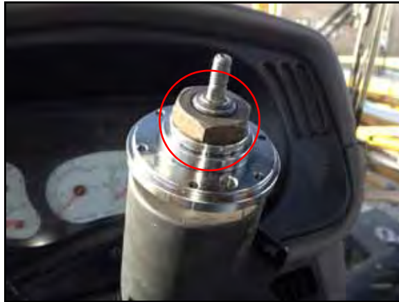
FIGURE 7. Machine's Steering Wheel Nut Installed
