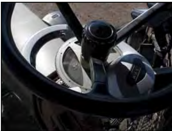
FIGURE 19. Mechanical Drive Installed
