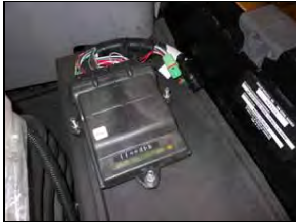
FIGURE 4. SmarTrax MD Node Installed
