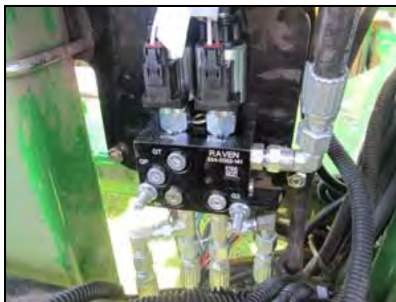
FIGURE 1. UltraGlide XT Valve Mounted to Existing Mounting Plate
