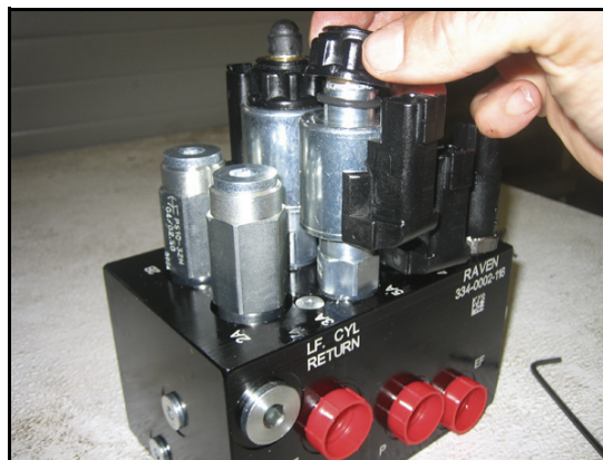
FIGURE 6. Coil Reinstalled on the AutoBoom Valve
