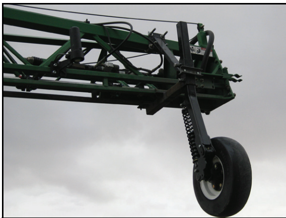
FIGURE 6. Gauge Wheel Installed
