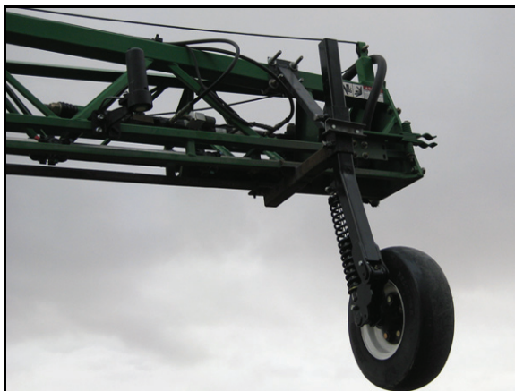
FIGURE 12. Gauge Wheel Installed
