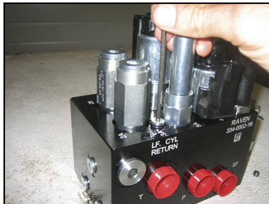
FIGURE 5. Port Plug Reinstalled on the AutoBoom Valve
