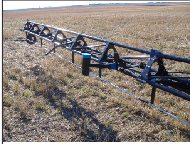
Mount sensor near boom tip.
