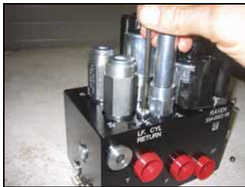
FIGURE 5. Port Plug Reinstalled on the AutoBoom Valve
