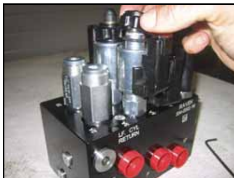
FIGURE 6. Coil Reinstalled on the AutoBoom Valve
