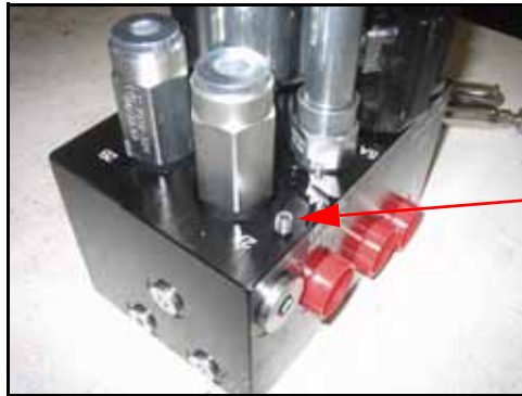
FIGURE 4. Orifice Fitting Removed from the AutoBoom Valve
