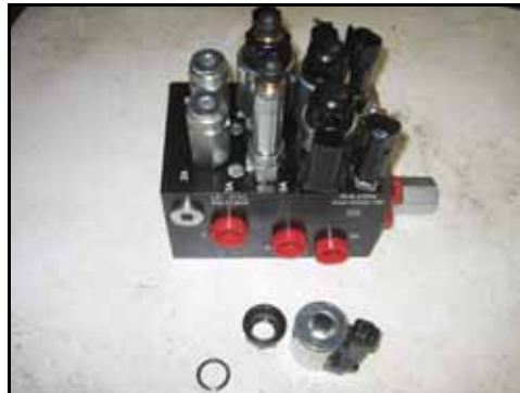
FIGURE 2. Coil Removed from the AutoBoom Valve
