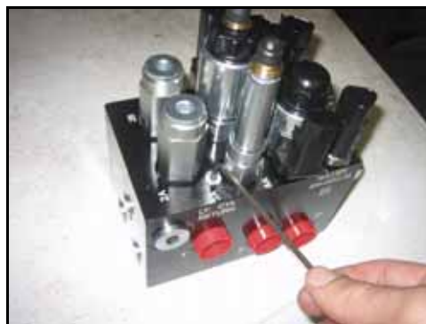
FIGURE 3. Port Plugs Removed from the AutoBoom Valve
