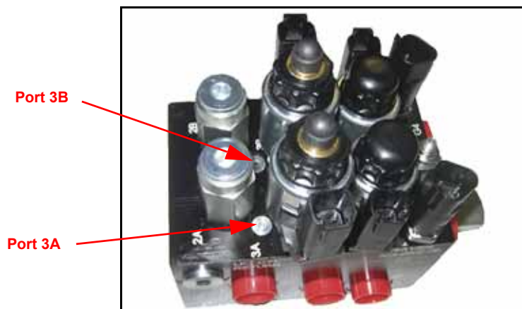
FIGURE 28. Port 3A and 3B Location
