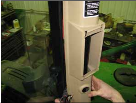
FIGURE 8. Post Cover Removed
