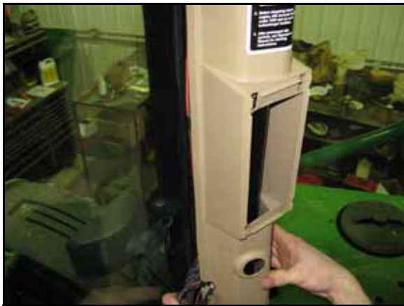
FIGURE 8. Post Cover Removed
