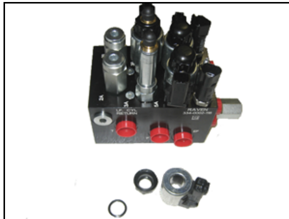
FIGURE 29. Coil Removed from the AutoBoom Valve
