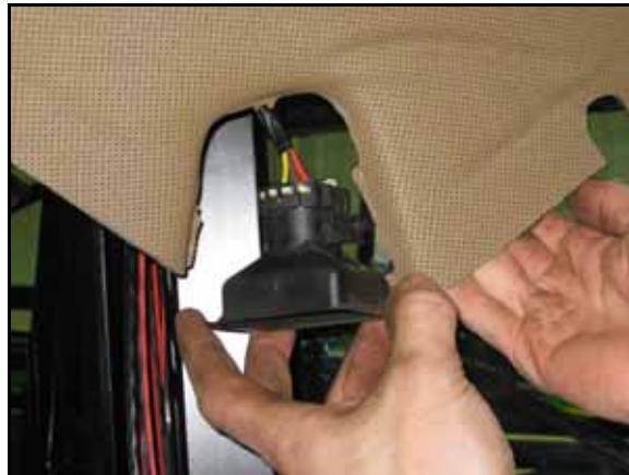
FIGURE 7. Terminator Removed from Harness Cable
