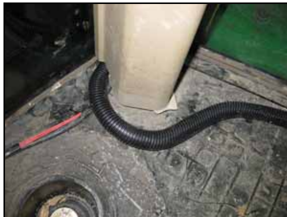
FIGURE 12. Post Cover Reinstalled Over the AutoBoom Harness Cable
