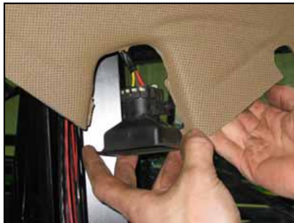
FIGURE 7. Terminator Removed from Harness Cable
