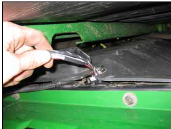
FIGURE 10. AutoBoom Harness Routed into the Machine's Cab
