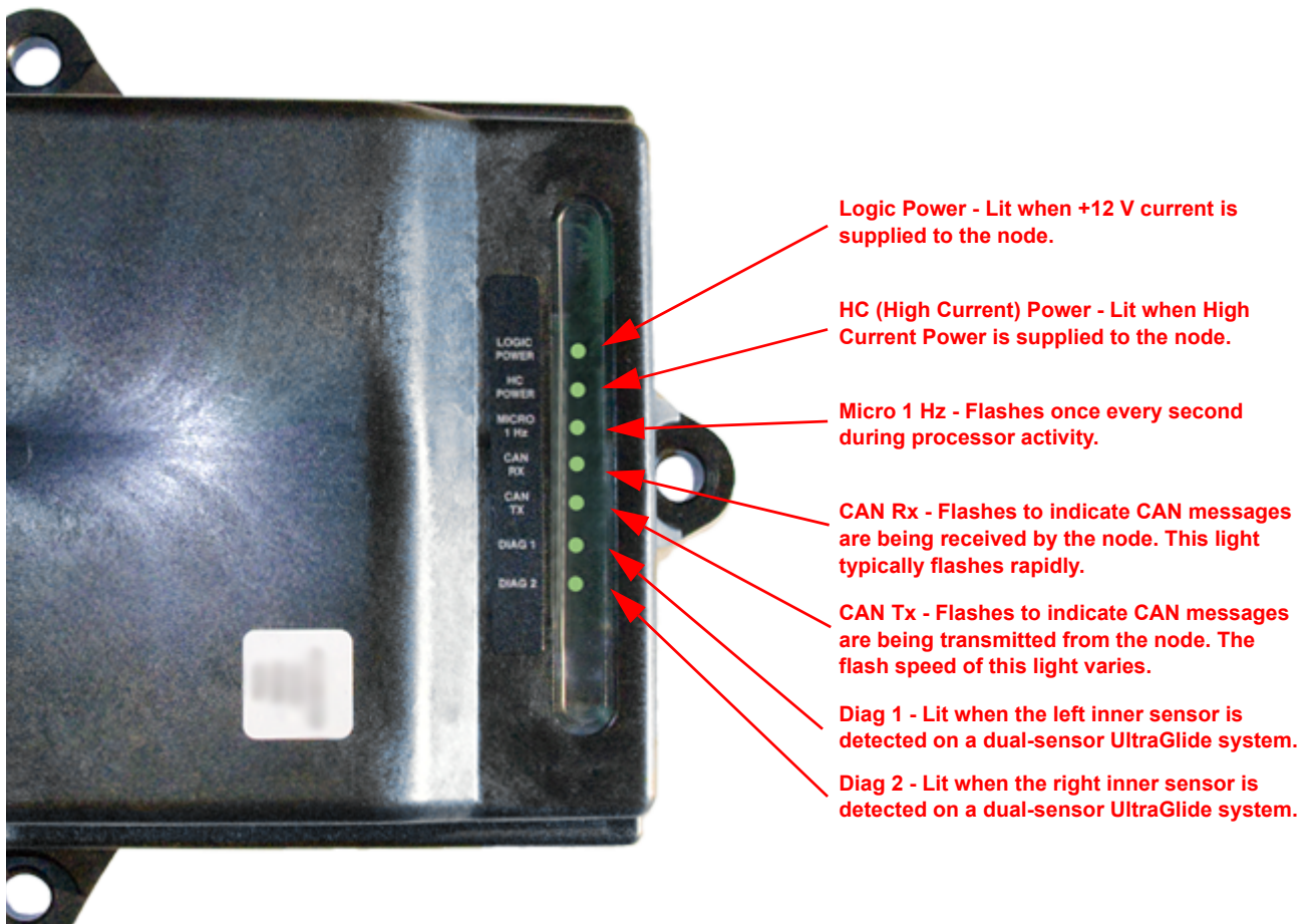
FIGURE 1. AutoBoom CAN Control Node LEDs
