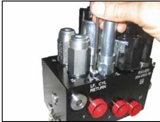
FIGURE 32. Port Plug Reinstalled on the AutoBoom Valve
