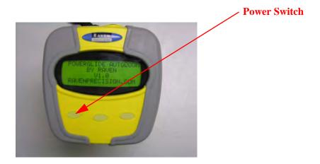
3. Enable the left and right booms with the controller by pressing the middle button for the left boom and the far right button for the right boom.
