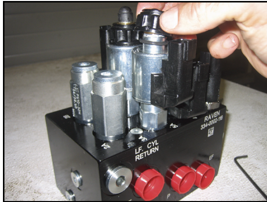
FIGURE 7. Coil Reinstalled on the AutoBoom Valve
