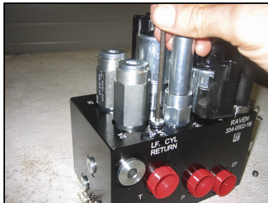
FIGURE 6. Port Plug Reinstalled on the AutoBoom Valve
