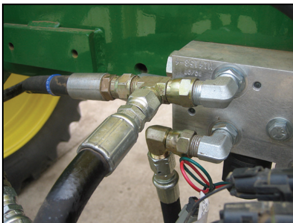
FIGURE 5. Pressure and Tank Hoses Installed
