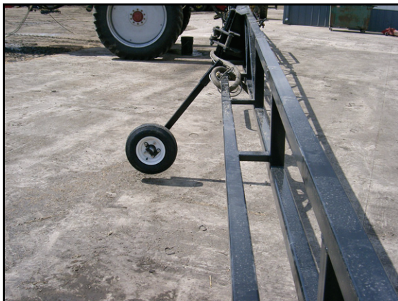
FIGURE 14. Gauge Wheel Installed
