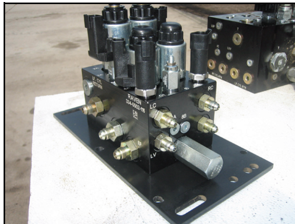
FIGURE 8. Fittings Installed on the AutoBoom Valve
