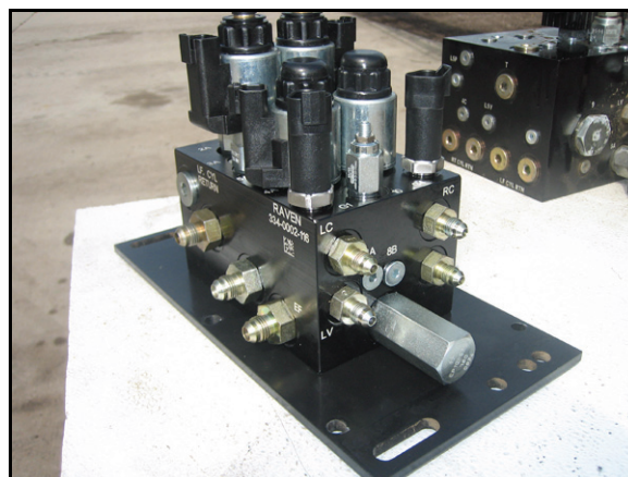
FIGURE 2. Fittings Installed on the AutoBoom Valve
