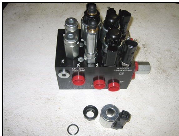
FIGURE 3. Coil Removed from the AutoBoom Valve
