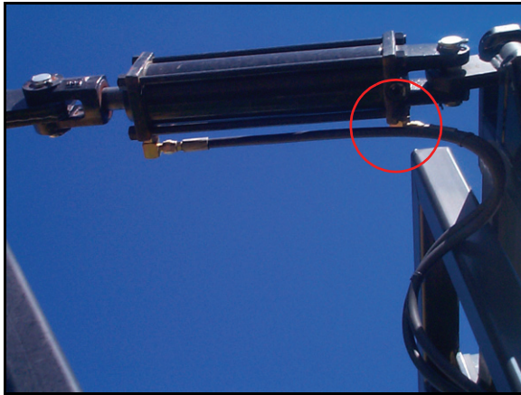
FIGURE 7. Down Hoses Installed
