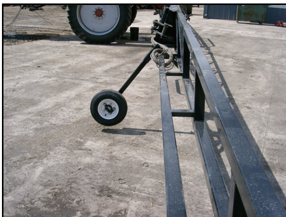
FIGURE 10. Gauge Wheel Installed
