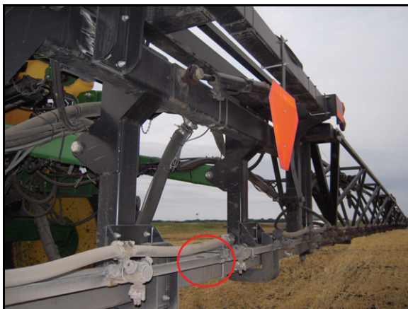
FIGURE 9. Center Rack Sensor Mounting Location
