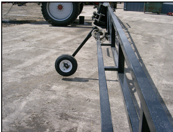
FIGURE 8. Gauge Wheel Installed
