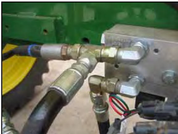
FIGURE 5. Pressure and Tank Hoses Installed
