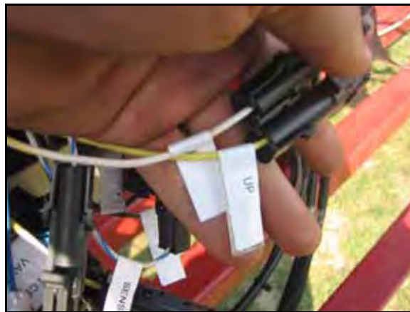
FIGURE 8. Machine's Up Cylinder Wiring
