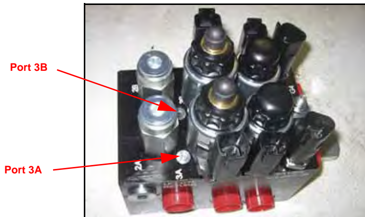
FIGURE 2. Port 3A and 3B Location
