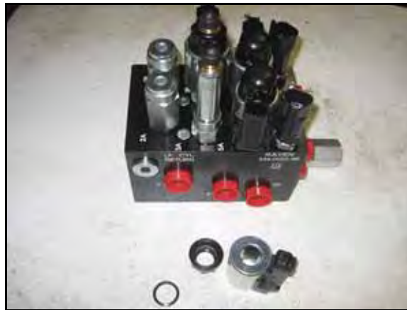
FIGURE 3. Coil Removed from the AutoBoom Valve
