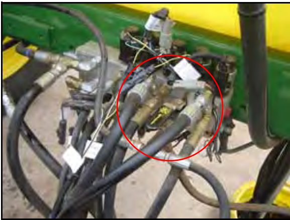
FIGURE 6. Left and Right Cylinder Hoses Installed
