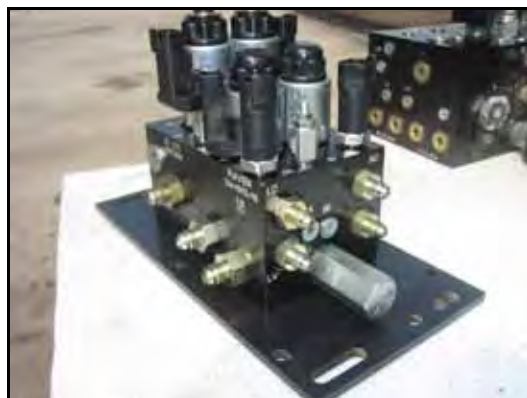
FIGURE 2. Fittings Installed on the AutoBoom Valve
