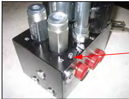
FIGURE 5. Orifice Fitting Removed from the AutoBoom Valve
