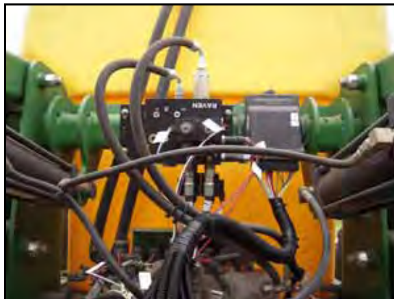
FIGURE 4. AutoBoom Valve Mounted to the Machine
