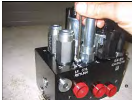
FIGURE 6. Port Plug Reinstalled on the AutoBoom Valve
