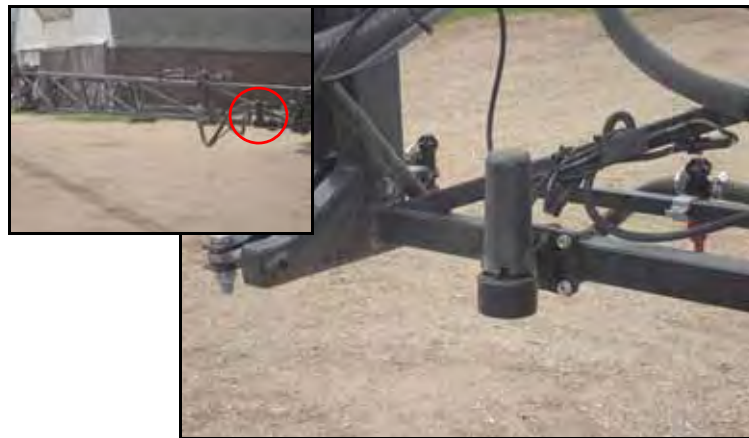
FIGURE 7. Mounted Boom Sensor
