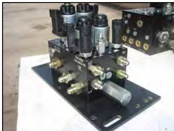
FIGURE 2. Fittings Installed on the AutoBoom Valve
