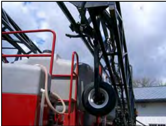
FIGURE 13. Gauge Wheel Installed
