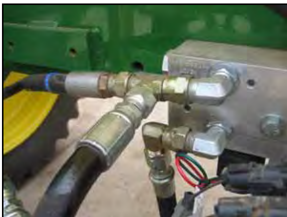
FIGURE 5. Pressure and Tank Hoses Installed
