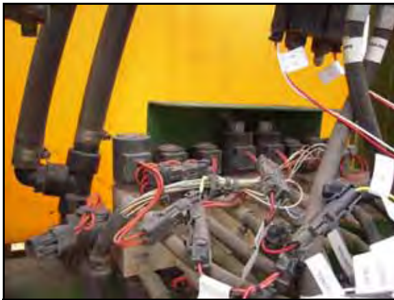
FIGURE 8. Machine's Up Cylinder Wiring
