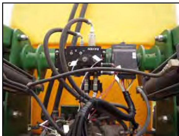
FIGURE 4. AutoBoom Valve Mounting Location
