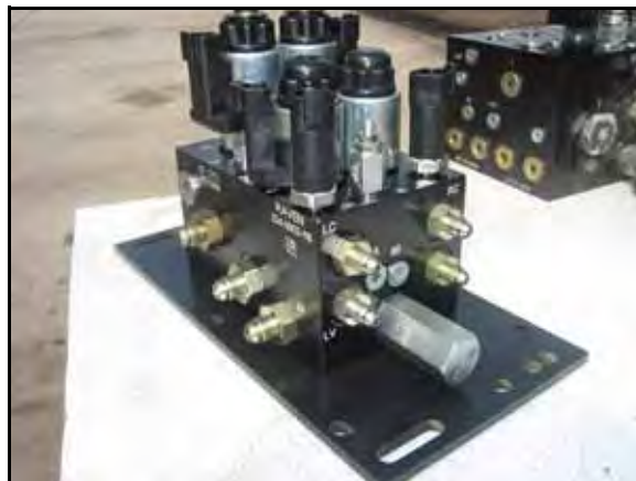
FIGURE 8. Fittings Installed on the AutoBoom Valve
