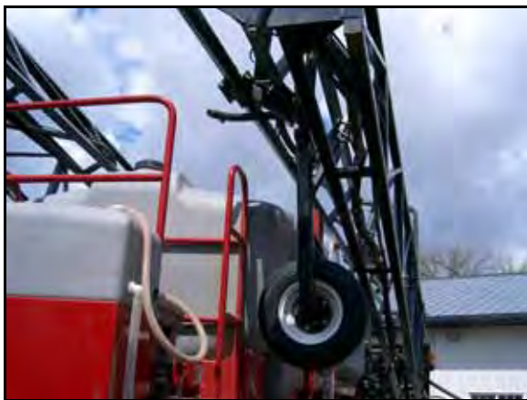
FIGURE 7. Gauge Wheel Installed
