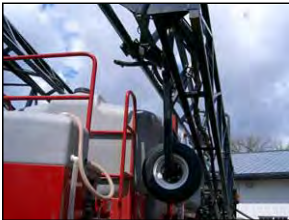
FIGURE 9. Gauge Wheel Installed
