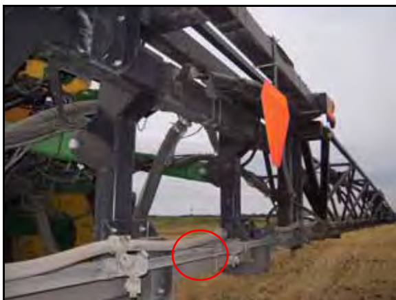
FIGURE 8. Mounted Center Rack Sensor
