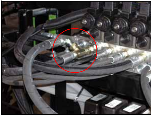
FIGURE 8. Left Cylinder Hose Installed
