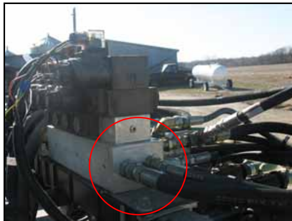
FIGURE 4. Pressure and Tank Hoses Installed on the Machine's Valve
