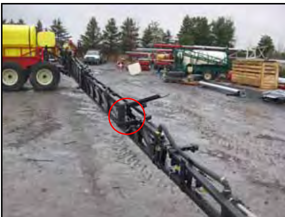
Outside Boom Sensor Mounting Location
