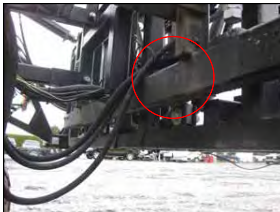
FIGURE 7. Center Rack Sensor Mounting Location
