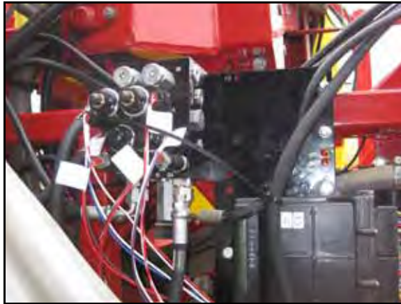
FIGURE 9. AutoBoom Valve Mounted to the Machine
