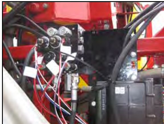
FIGURE 3. AutoBoom Valve Mounted to the Machine
