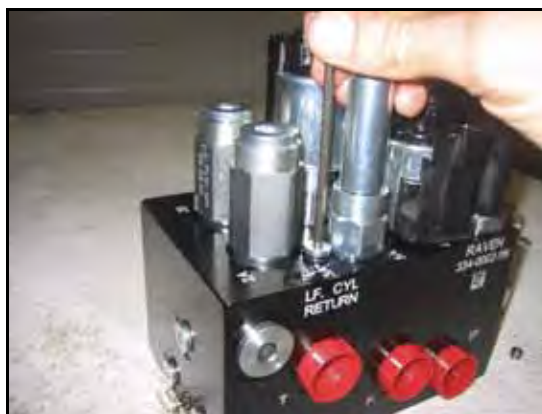
FIGURE 6. Port Plug Reinstalled on the AutoBoom Valve
