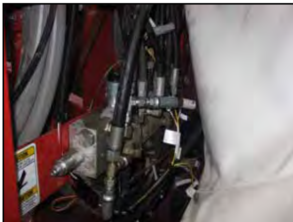
FIGURE 14. Directional Valve Boom Sense Adapter Cables Installed
