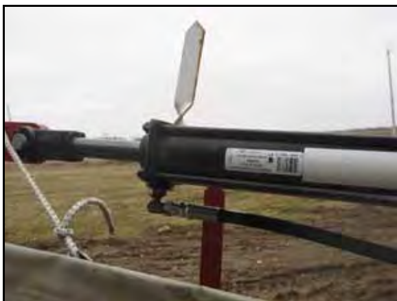
FIGURE 5. Cylinder Hoses Installed
