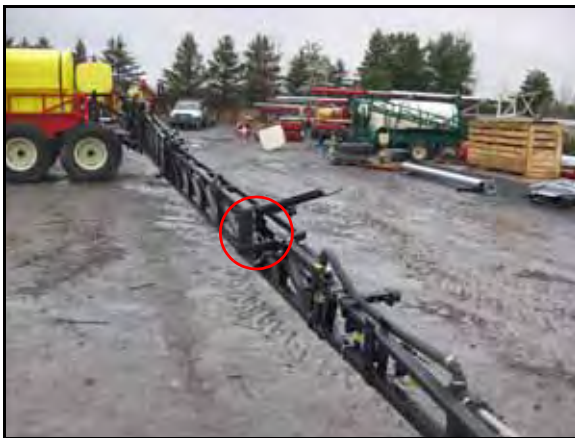
Outside Boom Sensor Mounting Location
