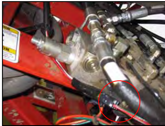
FIGURE 11. Directional Coil Boom Sense Adapter Cable Installed
