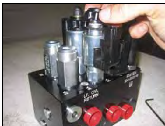
FIGURE 7. Coil Reinstalled on the AutoBoom Valve
