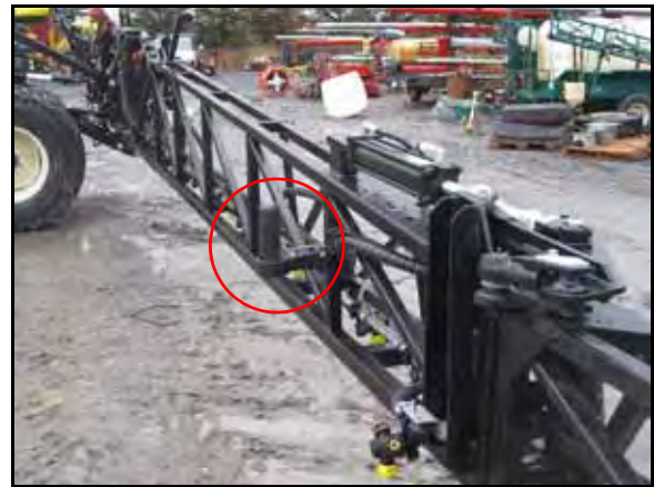
Optional Inside Boom Sensor Mounting Location
