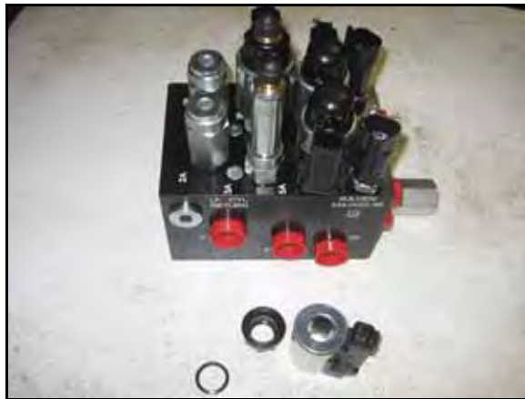
FIGURE 3. Coil Removed from the AutoBoom Valve
