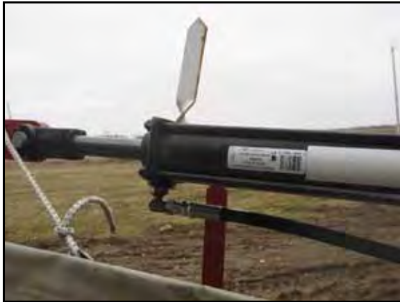
FIGURE 11. Cylinder Hoses Installed
