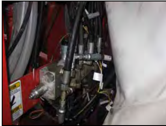
FIGURE 10. Boom Sense Adapter Cables Installed
