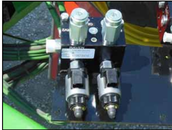
FIGURE 3. UltraGlide XT Valve Mounted on Valve Mounting Bracket
