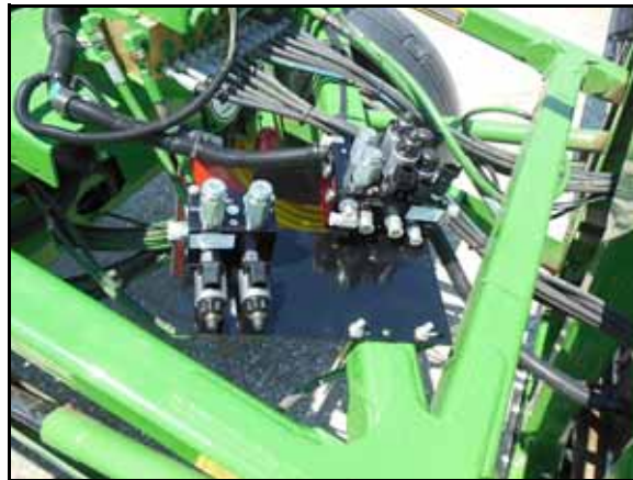
FIGURE 4. AutoBoom and UltraGlide XT Valves Mounted on the Machine
