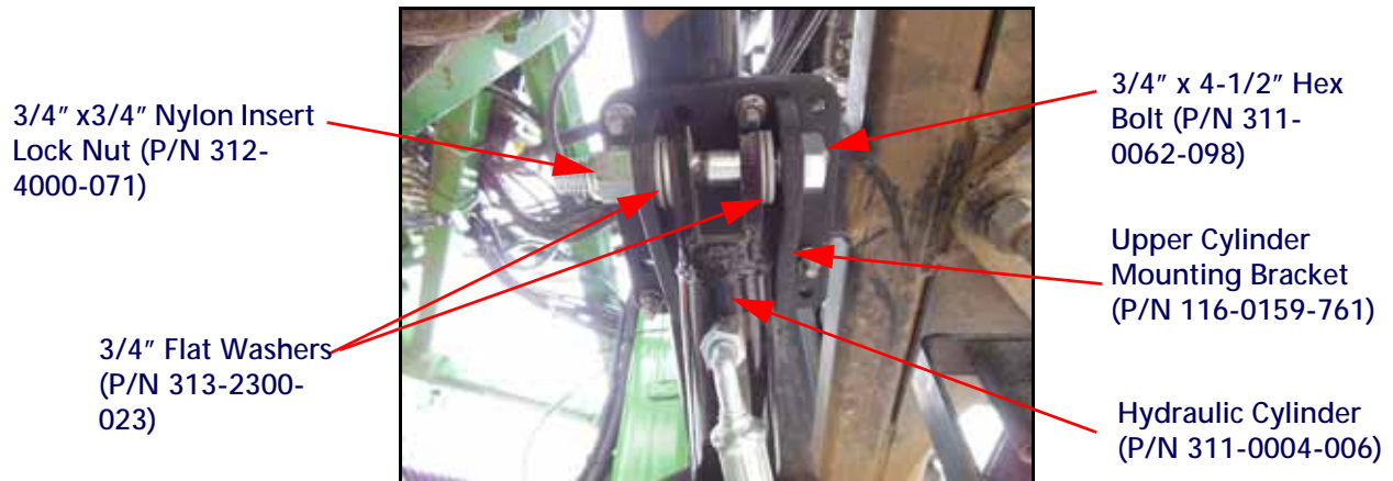
FIGURE 16. Base-End of Cylinder Installed on Upper Mounting Bracket
