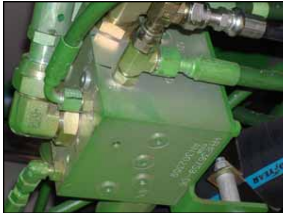
FIGURE 9. Load Sense Hose Connected to the Multi-Function Block
