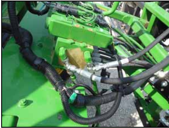
FIGURE 5. Pressure and Tank Hoses Installed on the Machine
