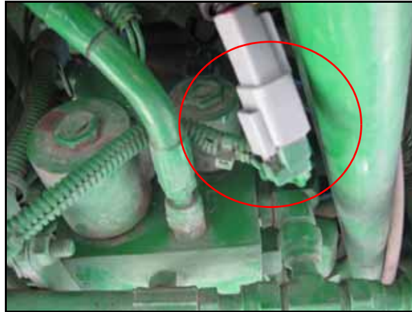
FIGURE 6. Load Sense Combo Valve Connection
