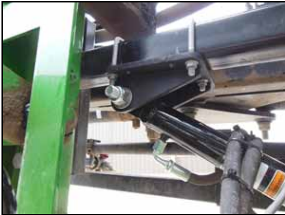
FIGURE 18. Right Hydraulic Cylinder Installed
