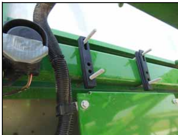
FIGURE 1. U-Bolts and Shims Installed
