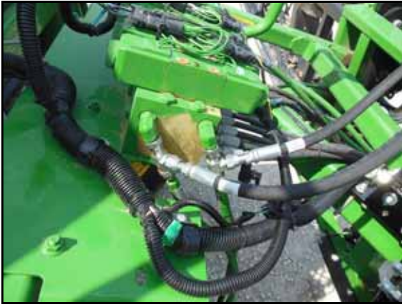
FIGURE 6. Pressure and Tank Hoses Installed on the Machine
