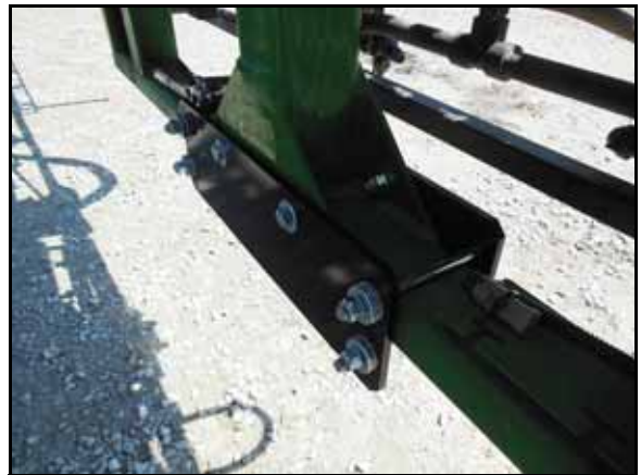
FIGURE 14. Cylinder Mount and Backing Plate Brackets Installed on Gusset Plates
