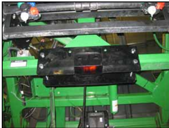
FIGURE 12. Lower Cylinder Mount and Backing Plate Brackets Installed
