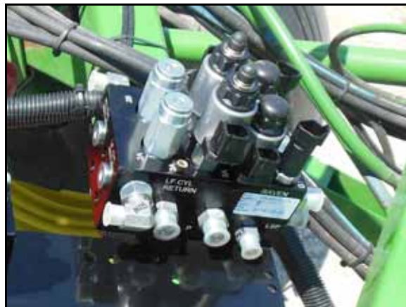
FIGURE 2. AutoBoom Valve Installed on Valve Mounting Bracket
