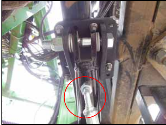
FIGURE 20. Cylinder Hose Installed on Hydraulic Cylinder
