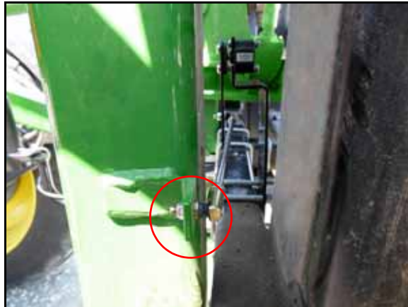
FIGURE 10. Installed Rotary Sensor Connection
