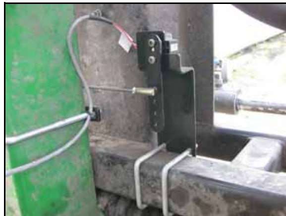
FIGURE 8. Rotary Sensor Mounting Bracket Installed
