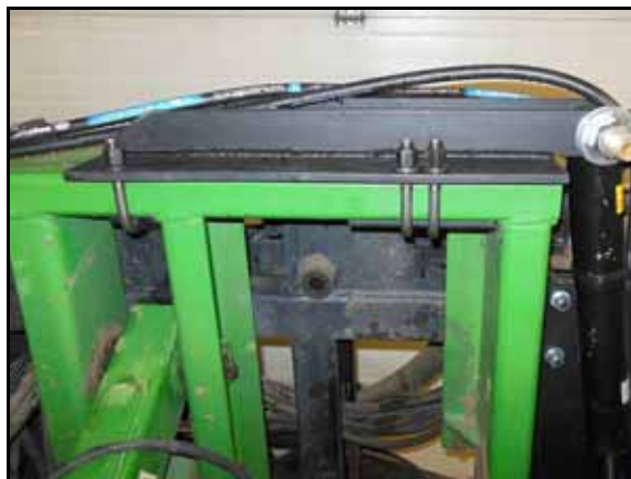
FIGURE 4. Upper Cylinder Mounting Bracket Installed
