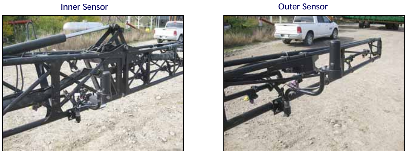
FIGURE 4. Boom Sensors Installed
