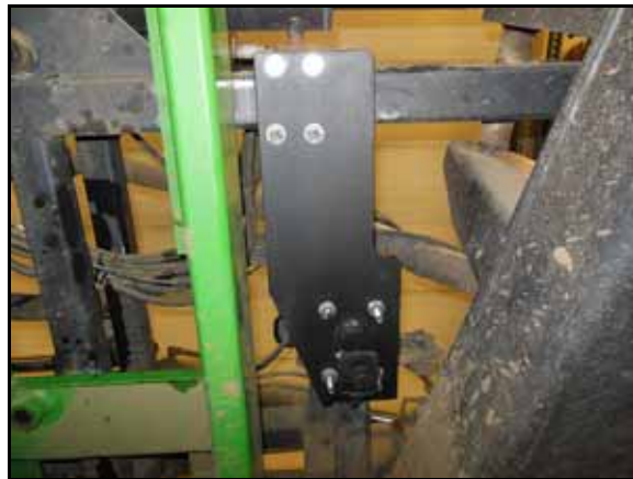
FIGURE 2. Left Lower Cylinder Mount Weldment Bracket Installed
