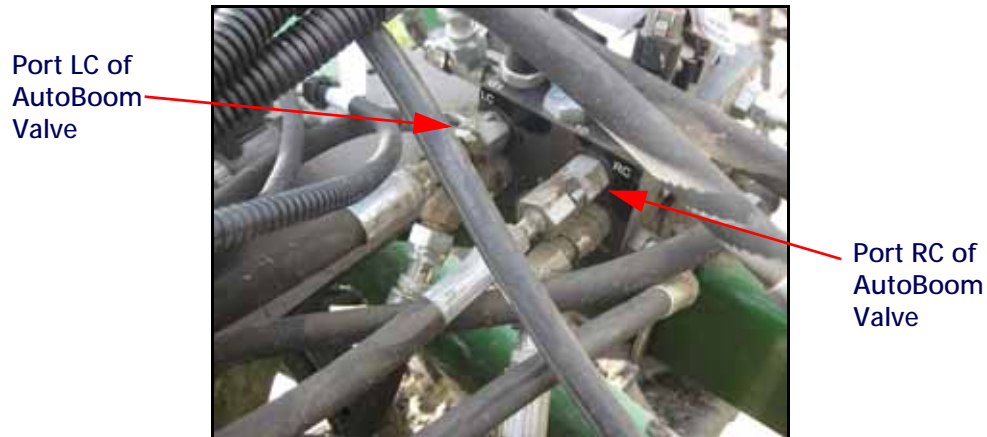
FIGURE 19. Left and Right Cylinder Hoses Installed
