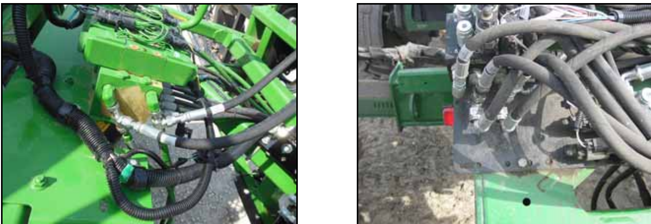
FIGURE 12. Pressure and Tank Hoses Installed on the Machine
