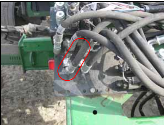
FIGURE 17. Hoses Installed on AutoBoom Hydraulic Valve
