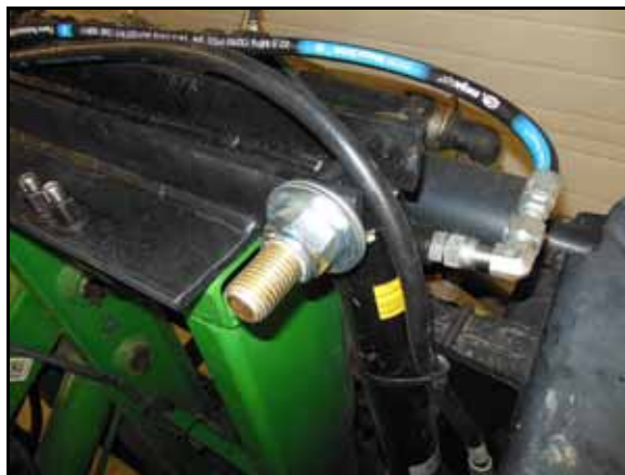
FIGURE 6. Base-End of Hydraulic Cylinder Installed
