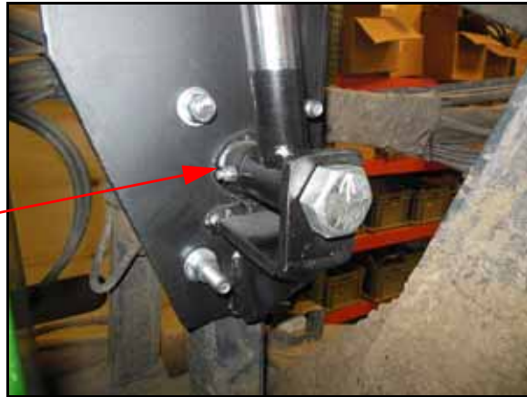
FIGURE 7. Rod-End of Hydraulic Cylinder Installed
