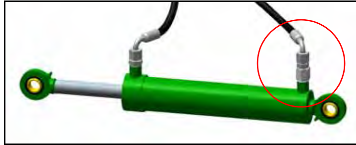
FIGURE 12. Base-End of Roll Bias Cylinder
