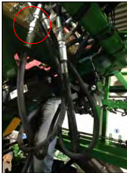
FIGURE 7. Hydraulic Hose Installed on Left Raise Hose
