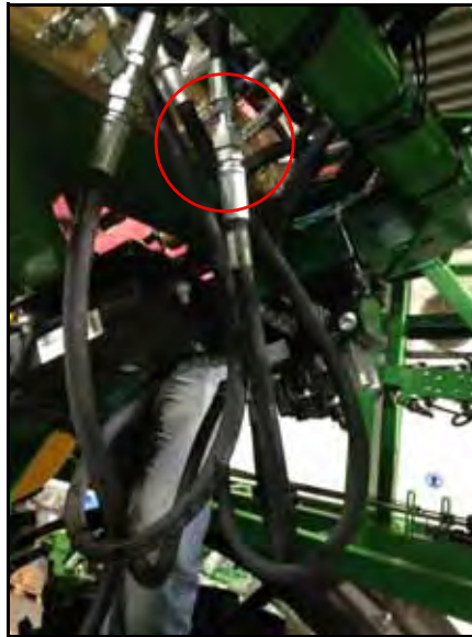
FIGURE 10. Hydraulic Hose Installed on Right Raise Hose
