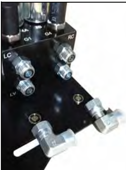
FIGURE 1. Fitting Installed in AutoBoom Valve
