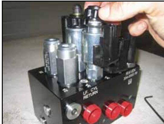
FIGURE 20. Coil Reinstalled on the AutoBoom Valve
