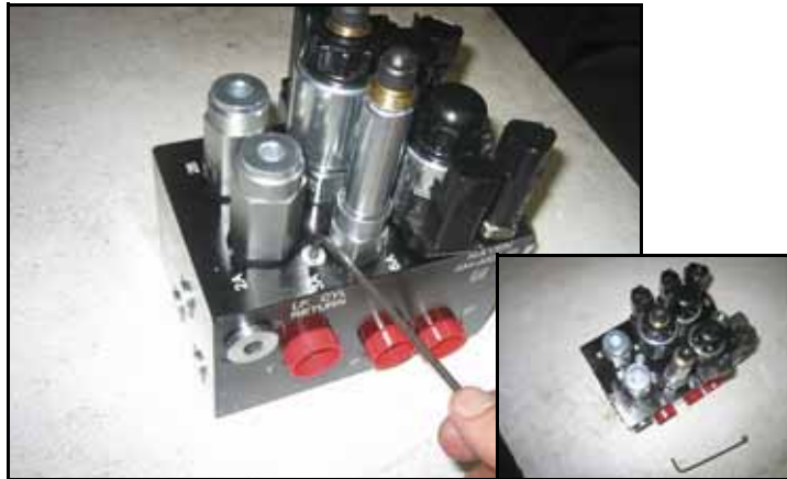
FIGURE 17. Port Plugs Removed from the AutoBoom Valve
