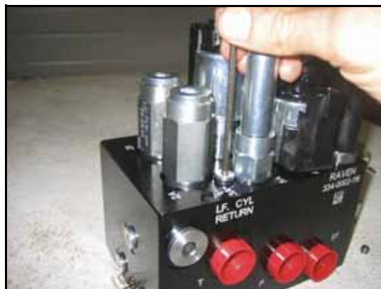
FIGURE 19. Port Plug Reinstalled on the AutoBoom Valve
