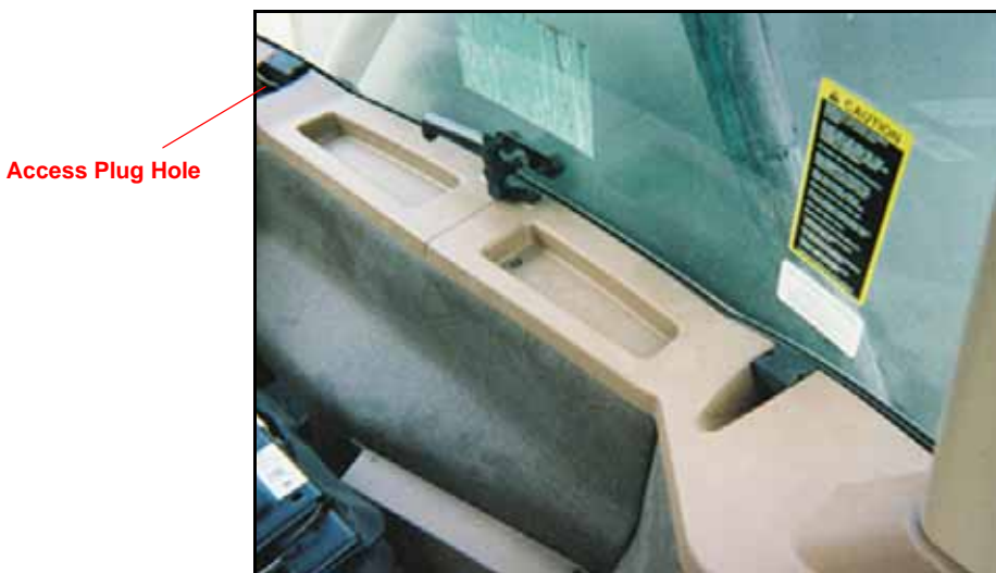
FIGURE 13. Access Plug Hole
