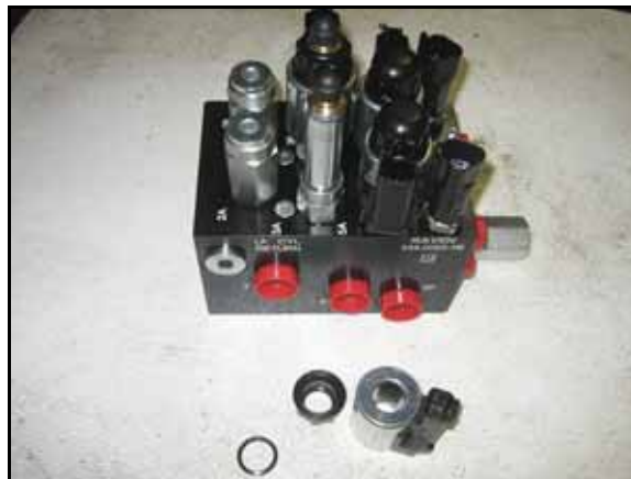
FIGURE 16. Coil Removed from the AutoBoom Valve
