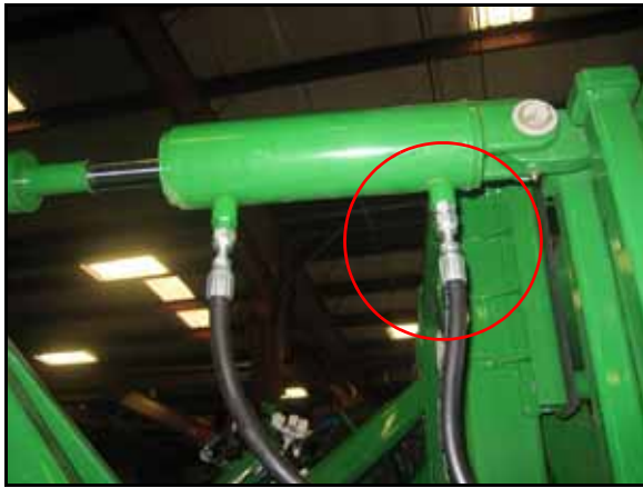
FIGURE 5. Down Hoses Installed
