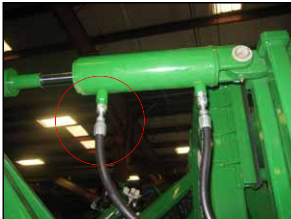
FIGURE 4. Cylinder Hoses Installed
