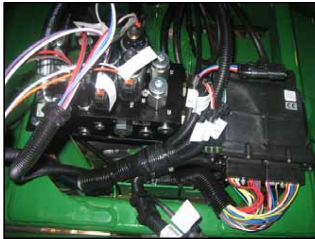
FIGURE 1. AutoBoom Valve Mounted on the Machine
