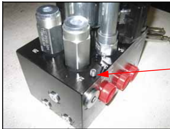
FIGURE 18. Orifice Fitting Removed from the AutoBoom Valve
