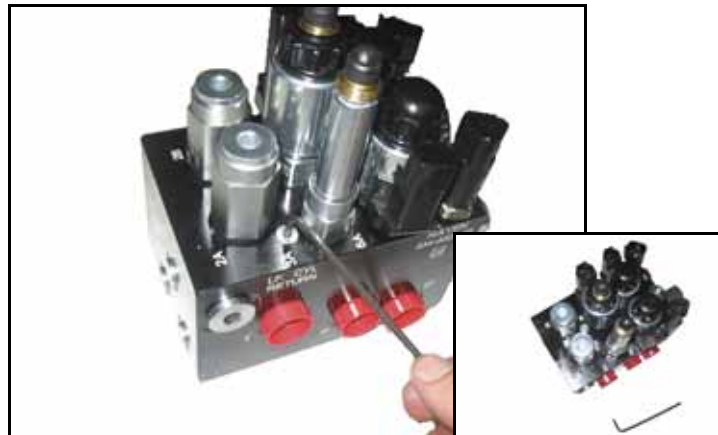
FIGURE 3. Port Plugs Removed from the AutoBoom Valve
