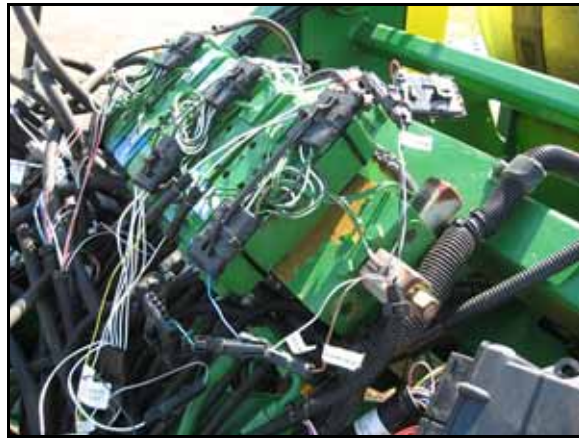
FIGURE 15. Machine's Center Rack Coils
