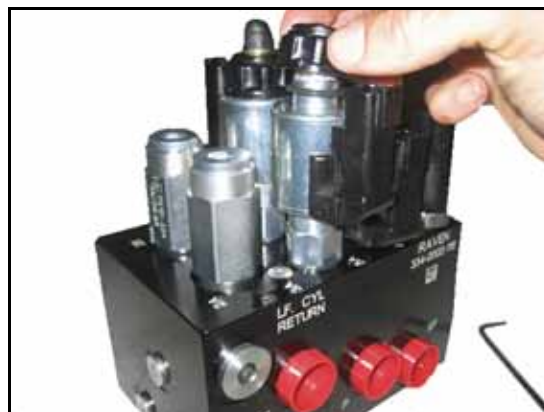
FIGURE 6. Coil Reinstalled on the AutoBoom Valve
