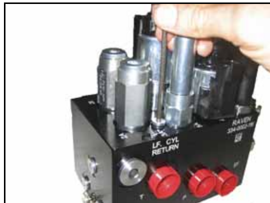
FIGURE 5. Port Plug Reinstalled on the AutoBoom Valve
