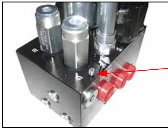
FIGURE 4. Orifice Fitting Removed from the AutoBoom Valve
