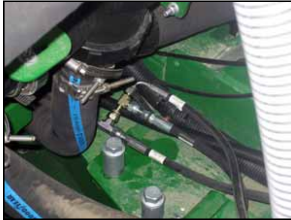
FIGURE 14. Load Sense Hose Installed
