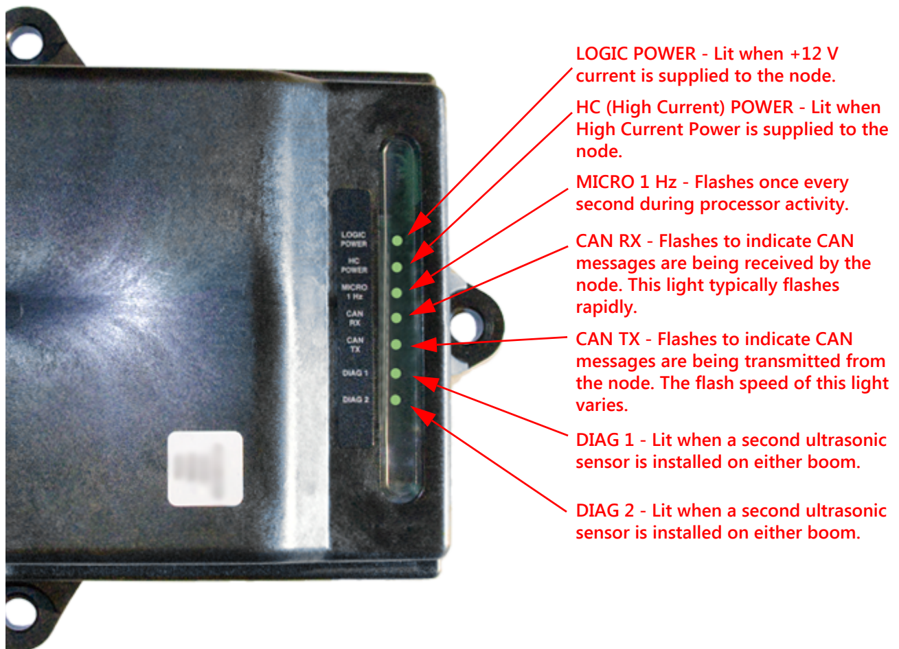
FIGURE 1. AutoBoom CAN Control Node LEDs
