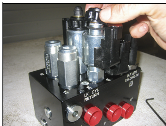
FIGURE 6. Coil Reinstalled on the AutoBoom Valve
