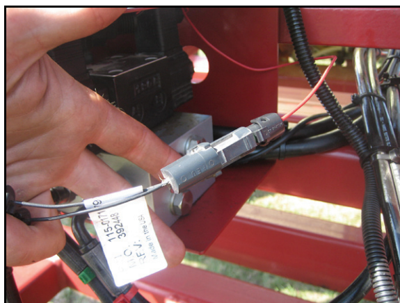
FIGURE 12. Single Weatherpack Boom Sense Adapter Cable Installed
