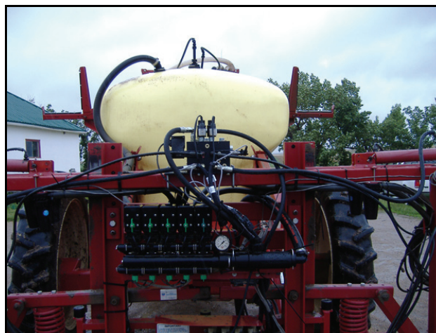
FIGURE 3. AutoBoom Valve Mounted to the Center Rack
