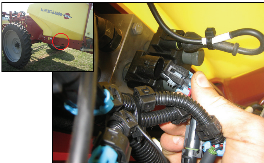
FIGURE 15. Center Rack Control Connections
