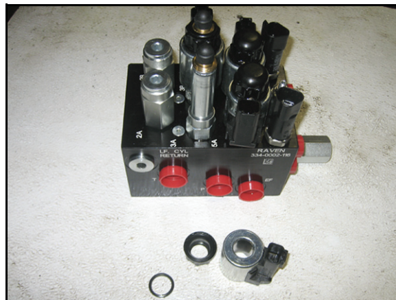
FIGURE 2. Coil Removed from the AutoBoom Valve
