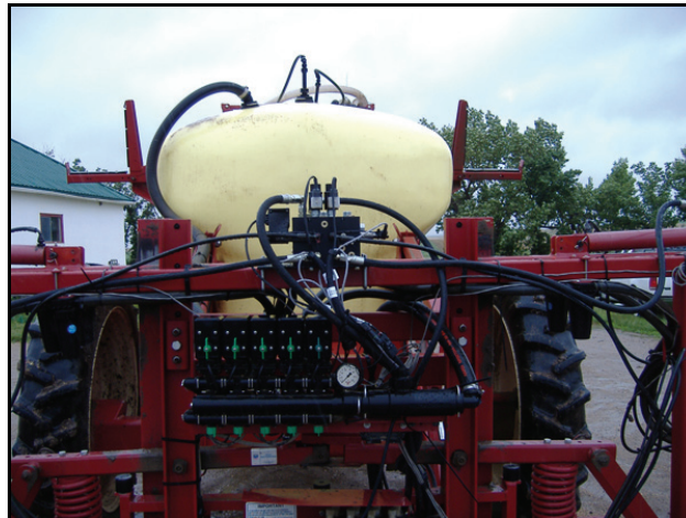
FIGURE 9. AutoBoom Valve Mounted to the Center Rack
