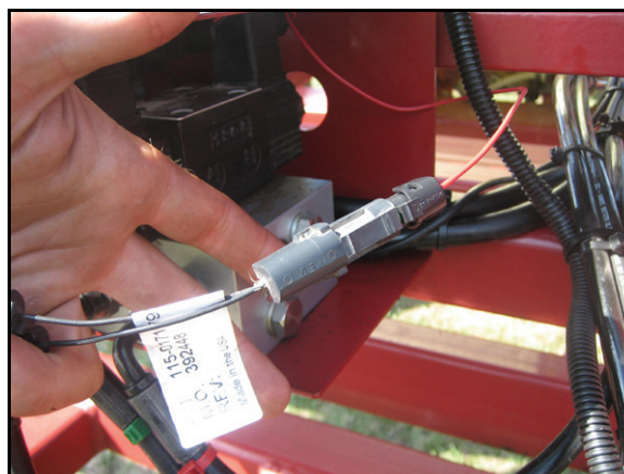
FIGURE 15. Single Weatherpack Boom Sense Adapter Cable Installed
