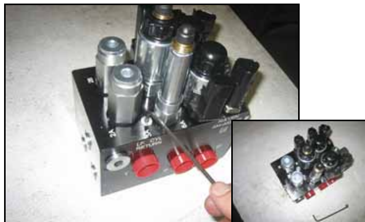
FIGURE 3. Port Plugs Removed from the AutoBoom Valve
