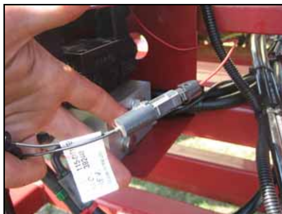
FIGURE 13. Single Weatherpack Boom Sense Adapter Cable Installed
