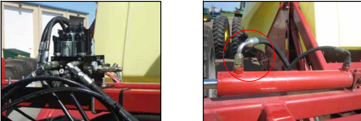
FIGURE 5. Cylinder Hoses Installed
