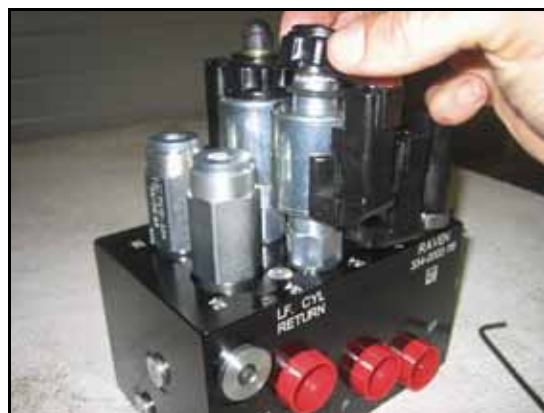
FIGURE 6. Coil Reinstalled on the AutoBoom Valve
