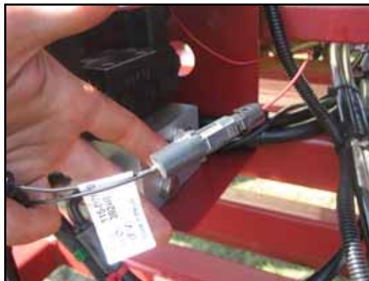
FIGURE 16. Single Weatherpack Boom Sense Adapter Cable Installed
