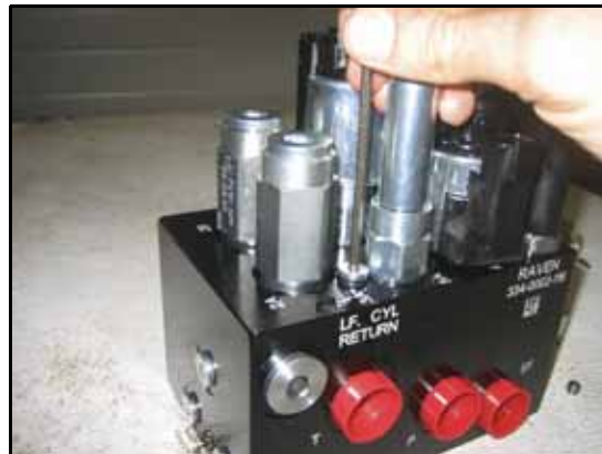
FIGURE 5. Port Plug Reinstalled on the AutoBoom Valve
