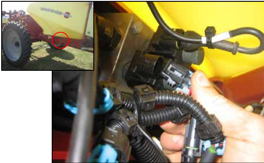
FIGURE 16. Center Rack Control Connections
