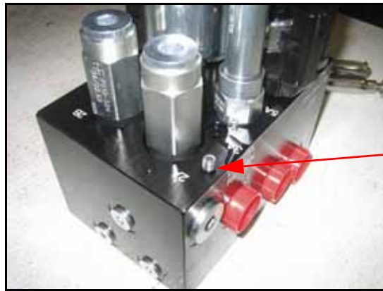
FIGURE 4. Orifice Fitting Removed from the AutoBoom Valve
