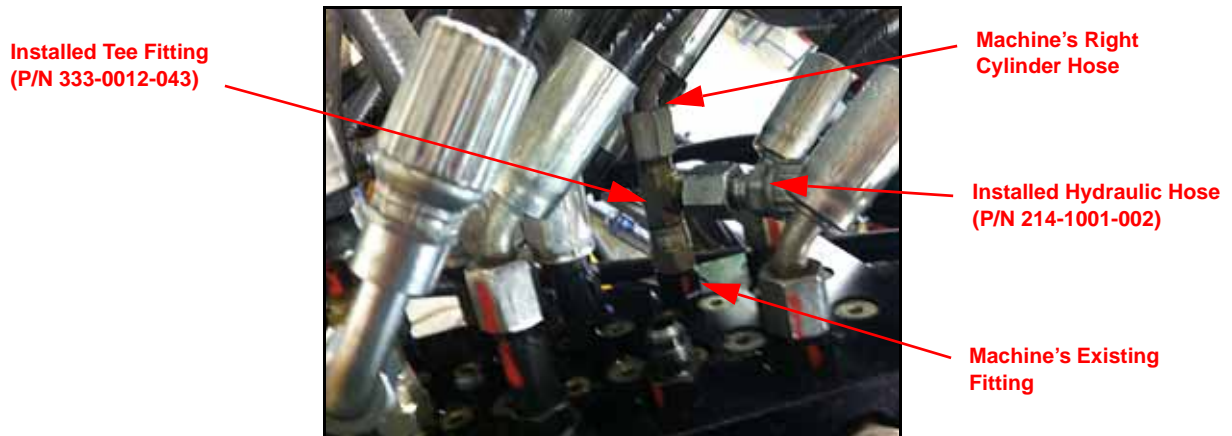
FIGURE 9. Right Cylinder Hose Installed on Cylinder
