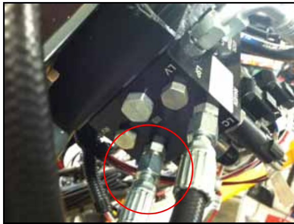
FIGURE 10. Right Cylinder Hose Installed on AutoBoom Valve
