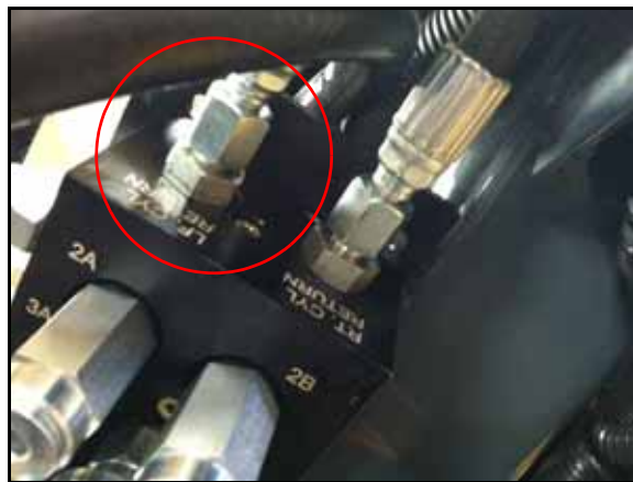
FIGURE 8. Left Cylinder Return Hose Installed on AutoBoom Valve
