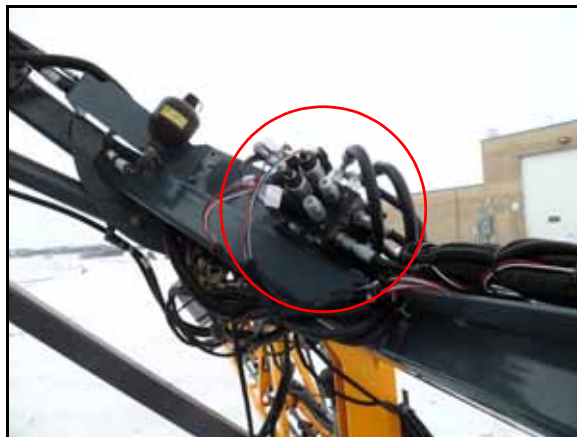
FIGURE 2. AutoBoom Valve Mounted on the Machine
