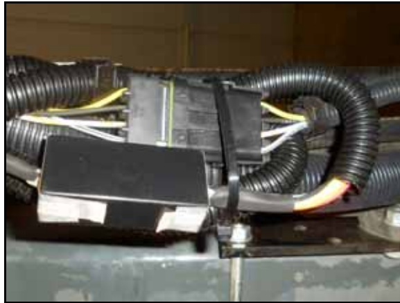
FIGURE 3. Serial Inverter Interface Installed on AutoBoom Harness
