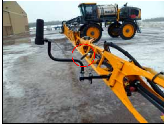
FIGURE 6. Harness Cable Connected to Sensor
