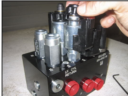
FIGURE 6. Coil Reinstalled on the AutoBoom Valve
