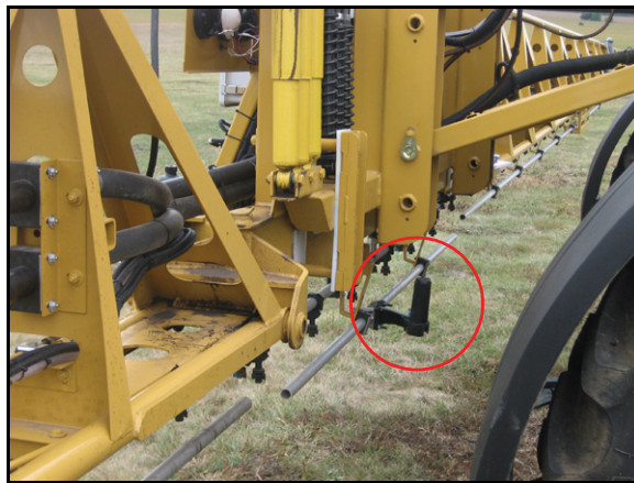
FIGURE 7. Mounted Center Rack Sensor
