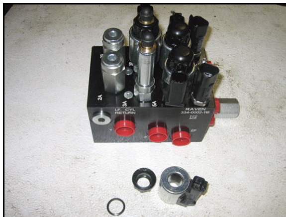
FIGURE 2. Coil Removed from the AutoBoom Valve
