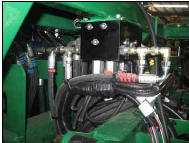
FIGURE 10. Left and Right Cylinder Down Hoses on the AutoBoom Valve (Dual Tilt Cylinder Option)
