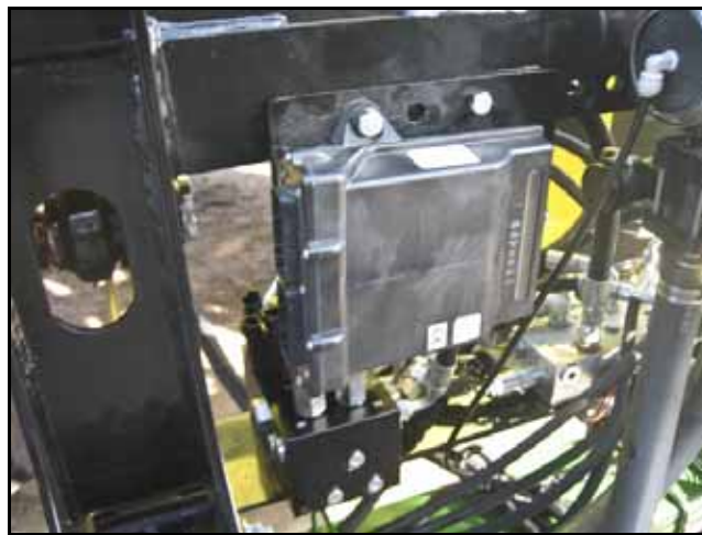
FIGURE 12. AutoBoom Node Installed
