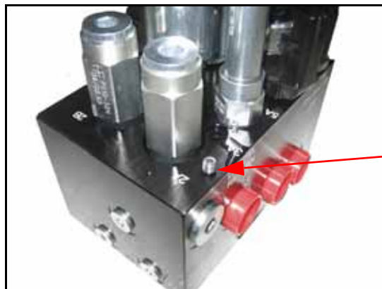
FIGURE 5. Orifice Fitting Removed from the AutoBoom Valve
