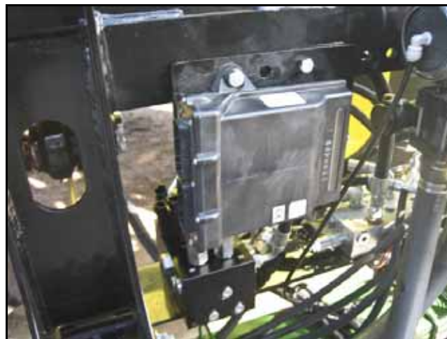
FIGURE 15. AutoBoom Node Installed
