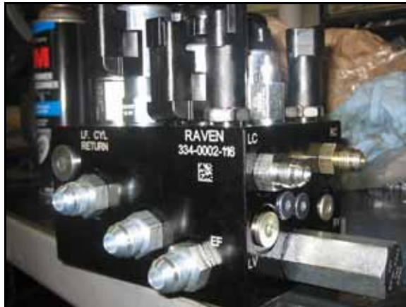
FIGURE 8. Fittings Installed on the AutoBoom Valve
