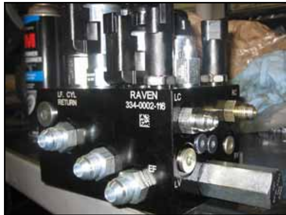
FIGURE 2. Fittings Installed on the AutoBoom Valve
