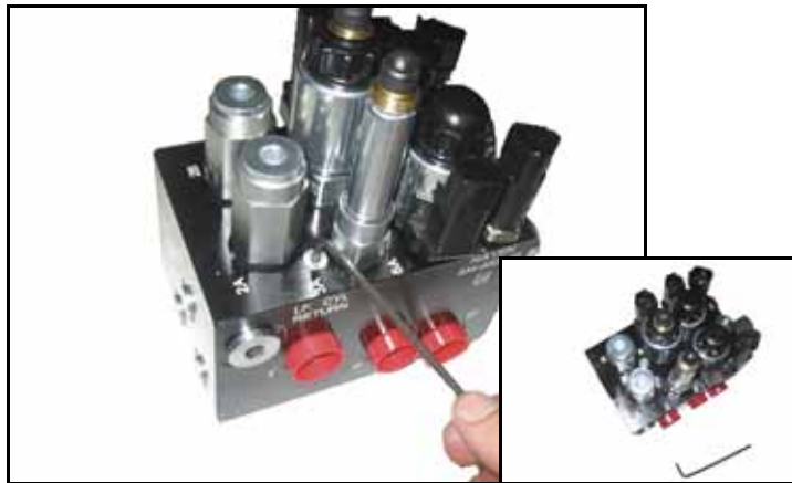
FIGURE 4. Port Plugs Removed from the AutoBoom Valve
