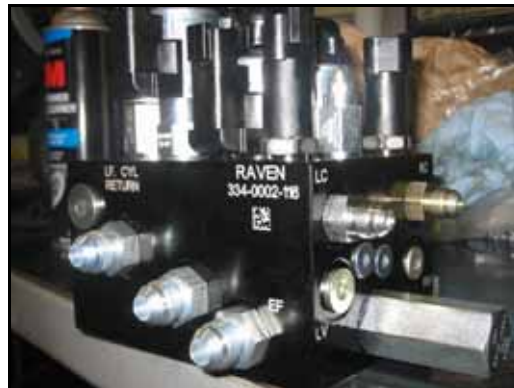
FIGURE 2. Fittings Installed on the AutoBoom Valve
