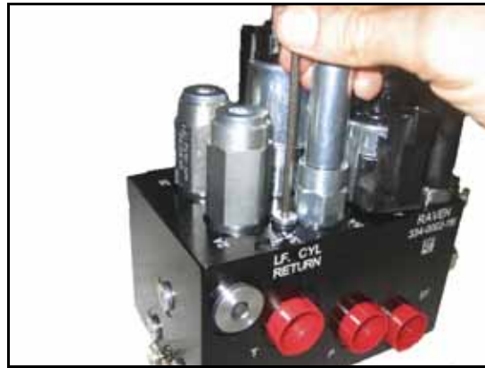
FIGURE 6. Port Plug Reinstalled on the AutoBoom Valve
