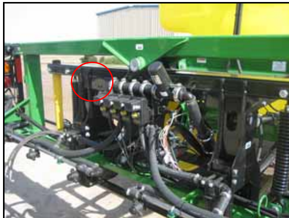
FIGURE 9. AutoBoom Valve Mounting Location
