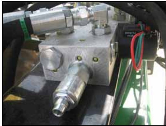
FIGURE 16. Machine's Directional Valve
