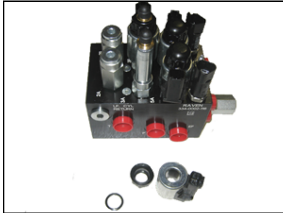
FIGURE 3. Coil Removed from the AutoBoom Valve
