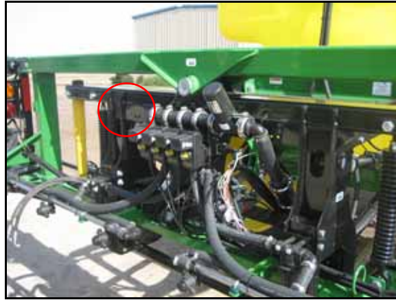
FIGURE 3. AutoBoom Valve Mounting Location
