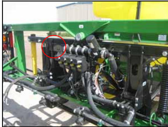
FIGURE 3. AutoBoom Valve Mounting Location
