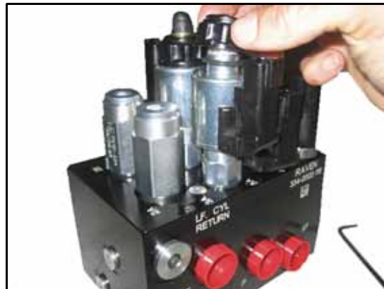
FIGURE 7. Coil Reinstalled on the AutoBoom Valve
