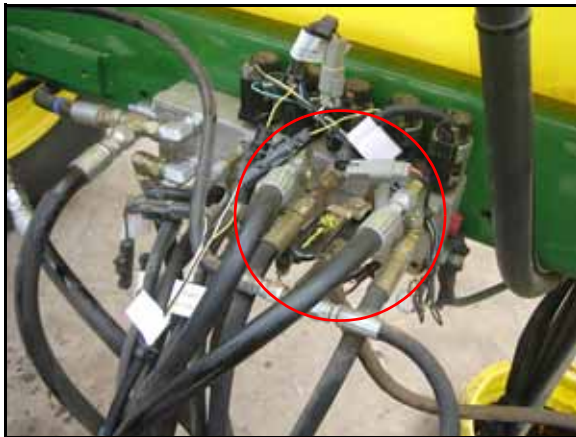
FIGURE 11. Cylinder Hoses Installed
