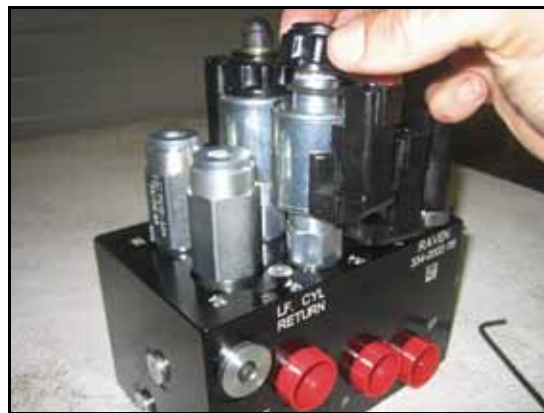
FIGURE 7. Coil Reinstalled on the AutoBoom Valve
