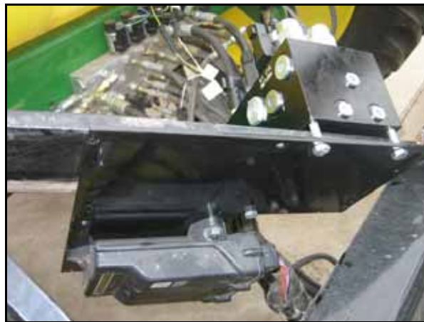
FIGURE 10. AutoBoom Node Installed
