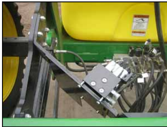
FIGURE 3. AutoBoom Valve Mounted on the Machine
