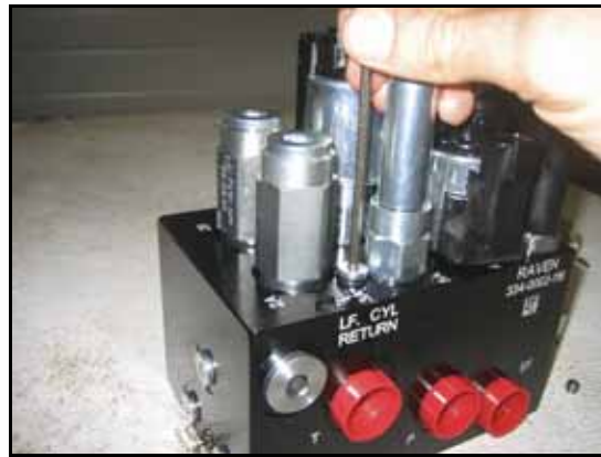
FIGURE 6. Port Plug Reinstalled on the AutoBoom Valve
