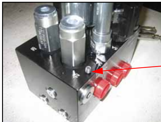
FIGURE 5. Orifice Fitting Removed from the AutoBoom Valve
