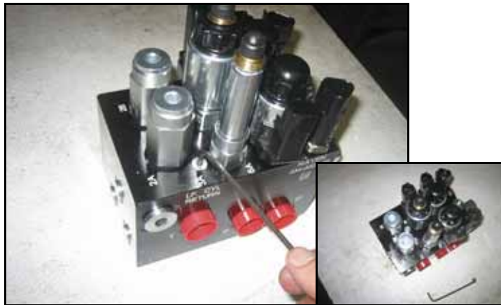
FIGURE 4. Port Plugs Removed from the AutoBoom Valve
