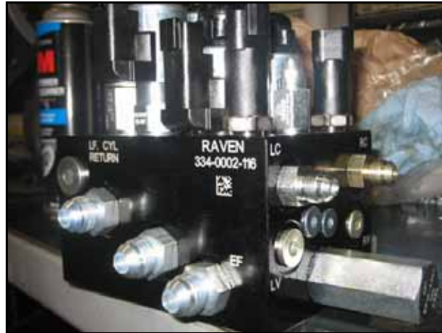
FIGURE 2. Fittings Installed on the AutoBoom Valve
