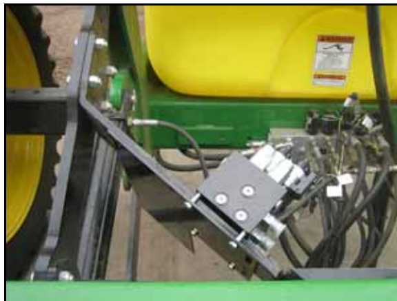
FIGURE 3. AutoBoom Valve Mounted on the Machine
