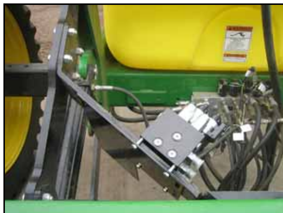
FIGURE 9. AutoBoom Valve Mounted on the Machine
