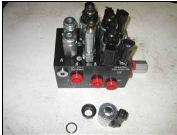
FIGURE 3. Coil Removed from the AutoBoom Valve
