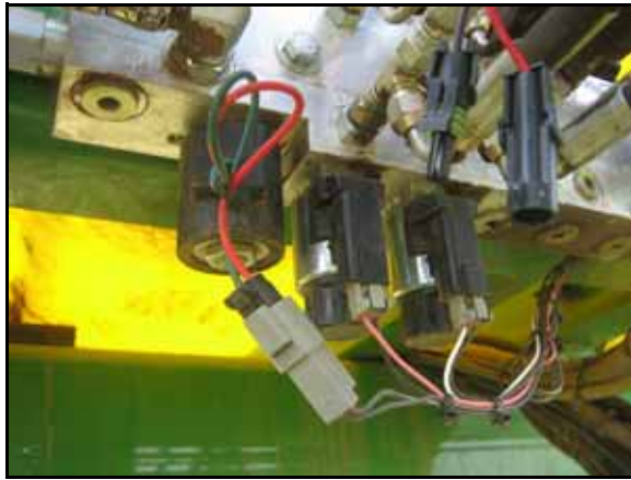
FIGURE 14. Directional Valve Boom Sense Adapter Cable Installed
