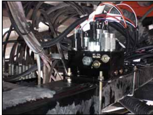
FIGURE 8. AutoBoom Valve Mounted to the Machine
