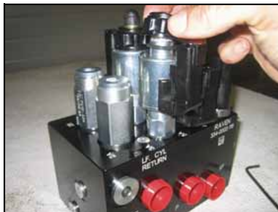
FIGURE 6. Coil Reinstalled on the AutoBoom Valve
