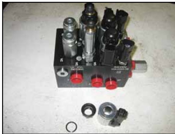
FIGURE 2. Coil Removed from the AutoBoom Valve
