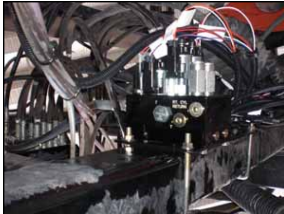
FIGURE 2. AutoBoom Valve Mounted to the Machine
