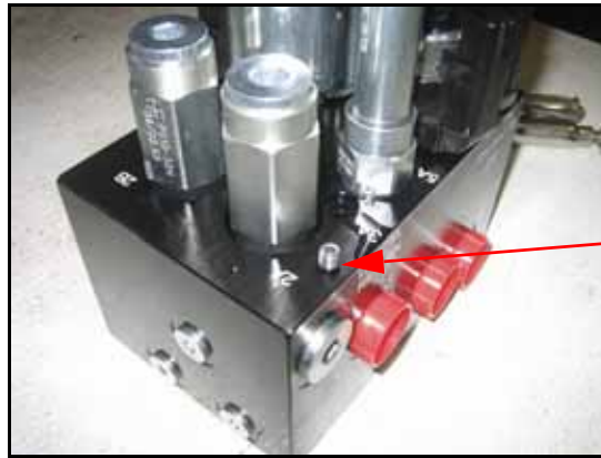
FIGURE 4. Orifice Fitting Removed from the AutoBoom Valve
