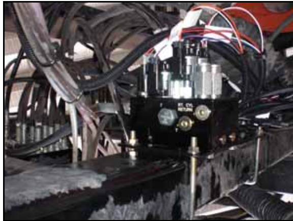
FIGURE 2. AutoBoom Valve Mounted to the Machine
