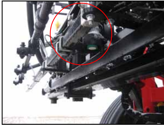
FIGURE 7. Mounted Center Rack Sensor
