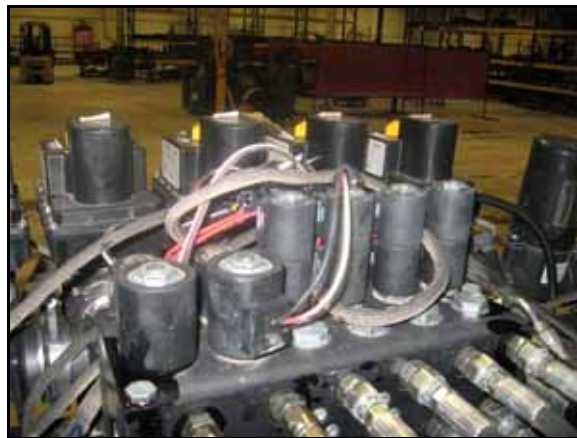
FIGURE 6. Machine's Left and Right Boom Function Controls
