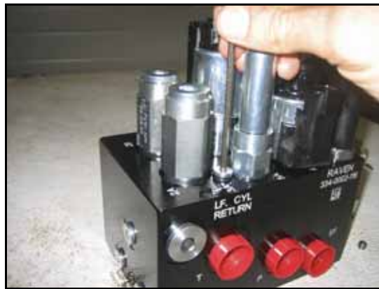
FIGURE 5. Port Plug Reinstalled on the AutoBoom Valve
